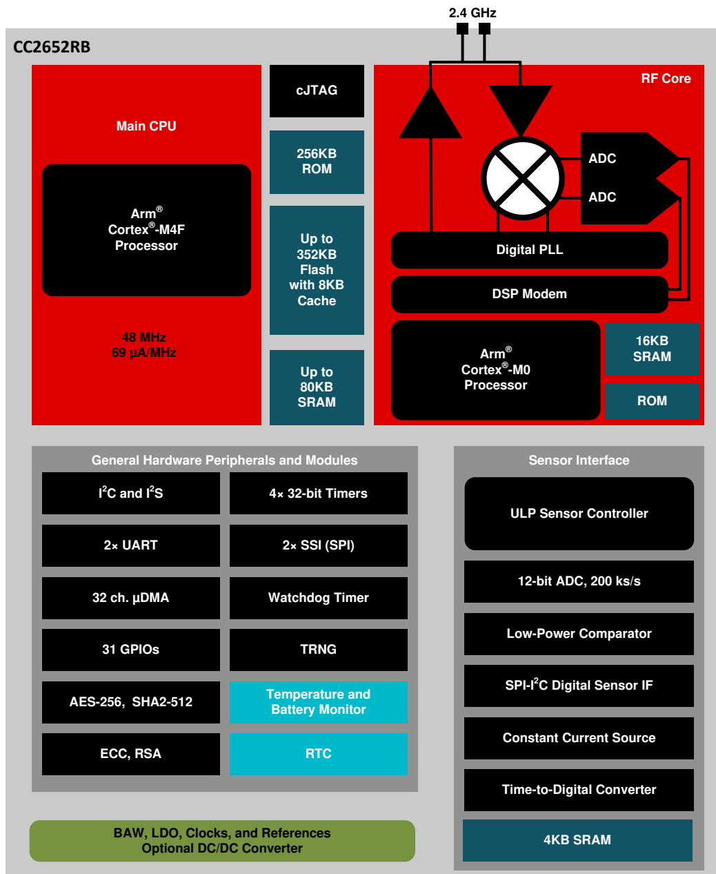
Figure 4-1. CC2652RB Block Diagram
