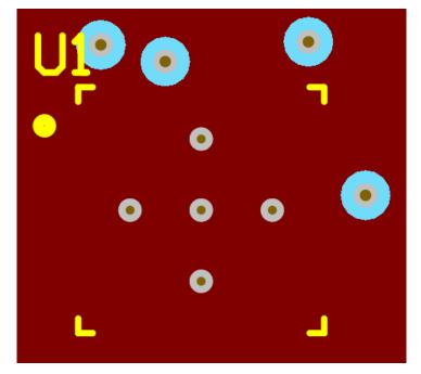
Figure 11-2. PCB Layout Example for CDCDB400, GND Layer
