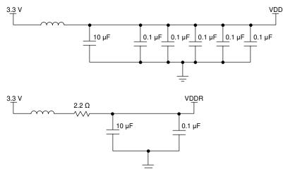
Figure 10-1. Power Supply Decoupling
