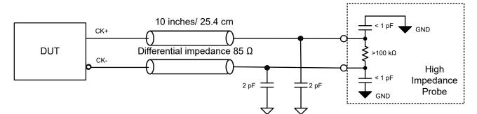
Figure 7-1. AC Test Load (Referencing Intel DB2000QL Document)
