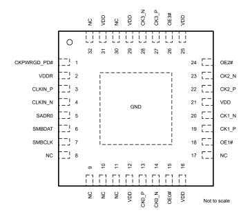
Figure 5-1. CDCDB400 RHB Package 32-Pin VQFN Top View
