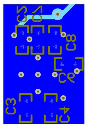
Figure 11-3. PCB Layout Example for CDCDB400, Bottom Layer
