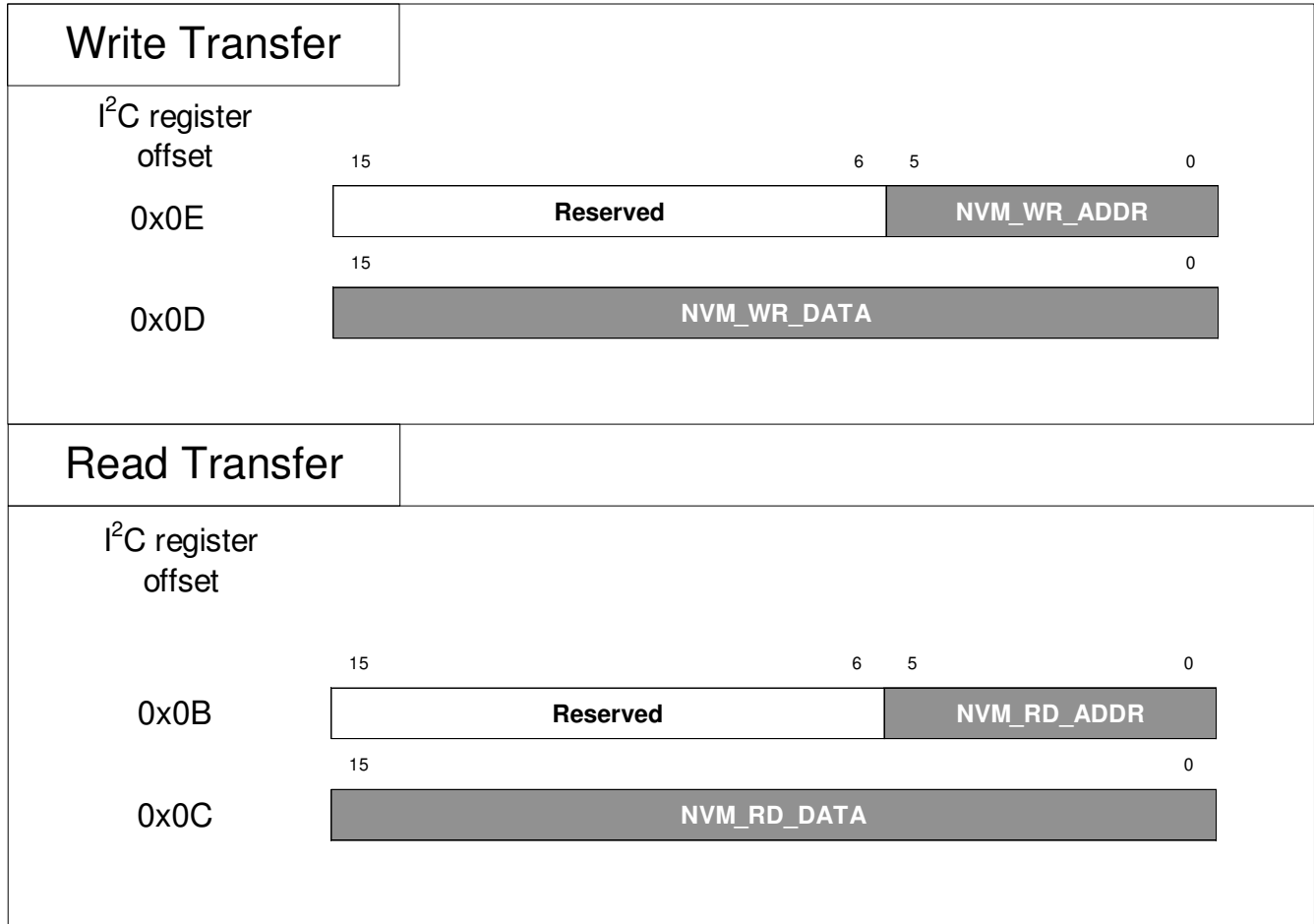
Figure 9-12. EEPROM Direct Access Using I 2 C
