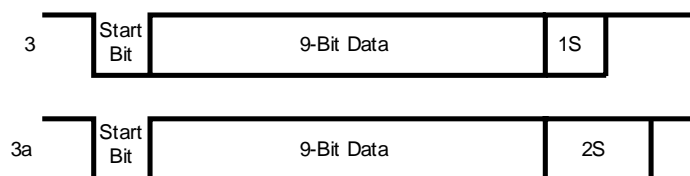
Figure 27-6. . 9-bit Data Frame Options
