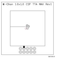
Max  $R_{\theta JA} = 131.1^{\circ}$ C/W when mounted on 1 inch<sup>2</sup> of 2 oz. Cu.
