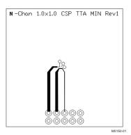
Max  $R_{\theta JA} = 228.6$  °C/W when mounted on minimum pad area of 2 oz. Cu.
