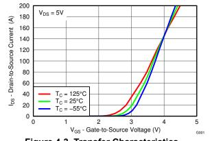
Figure 4-3. Transfer Characteristics
