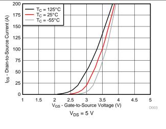
Figure 3. Transfer Characteristics
