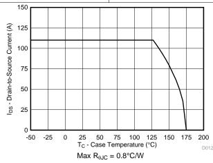
Figure 12. Maximum Drain Current vs Temperature
