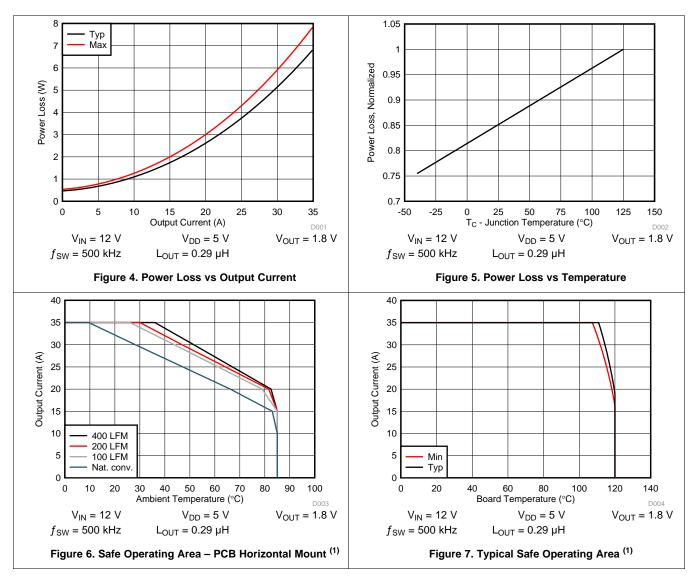
1. The typical CSD95377Q4M system characteristic curves are based on measurements made on a PCB design with dimensions of 4 in (W) × 3.5 in (L) × 0.062 in (T) and 6 copper layers of 1-oz copper thickness. See *System Example* for detailed explanation.
