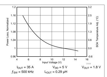
Figure 9. Normalized Power Loss vs Input Voltage
