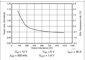
Figure 11. Normalized Power Loss vs Output Inductance
