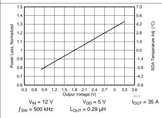
Figure 10. Normalized Power Loss vs Output Voltage
