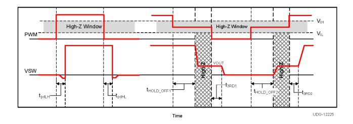
Figure 2. PWM Tri-State Timing Diagram
