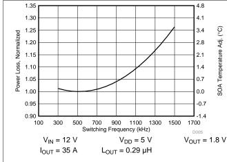
Figure 8. Normalized Power Loss vs Frequency
