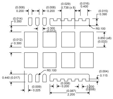
NOTE: Dimensions are in mm (in). Stencil is 100-µm thick.
