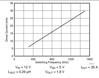
Figure 12. Driver Current vs Frequency
