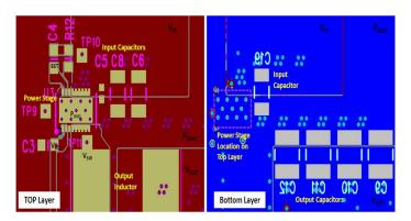
Figure 16. Recommended PCB Layout (Top-Down View)
