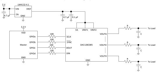
Figure 32. The LM4132 as a Power Supply
