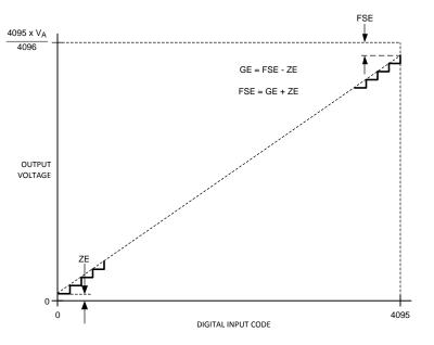
Figure 31. Input / Output Transfer Characteristic
