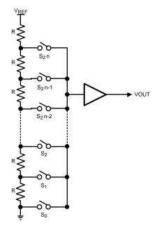
Figure 26. DAC Resistor String
