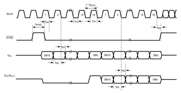
Figure 1. Serial Timing Diagram
