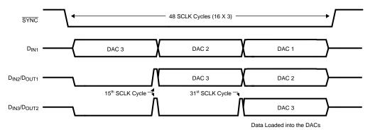
Figure 30. Daisy Chain Timing Diagram
