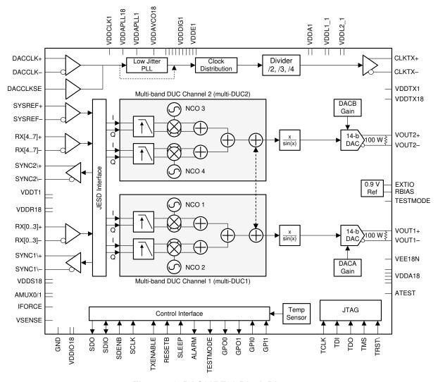
Figure 7-2. DAC38RF83 Block Diagram
