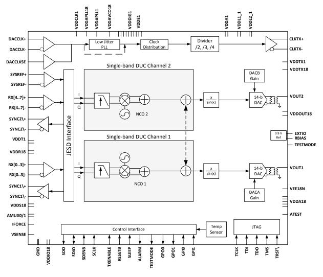
Figure 7-5. DAC38RF90 Block Diagram
