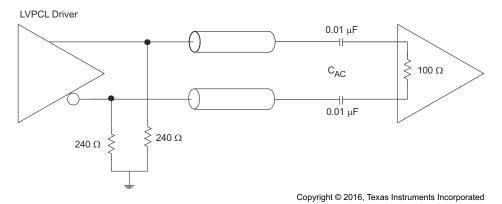
Figure 7-25. Preferred Clock Input Configuration With a Differential ECL/PECL Clock Source
