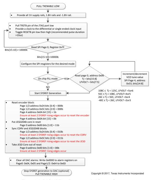
Figure 8-1. DAC38RF8xx Recommended Startup Sequence
