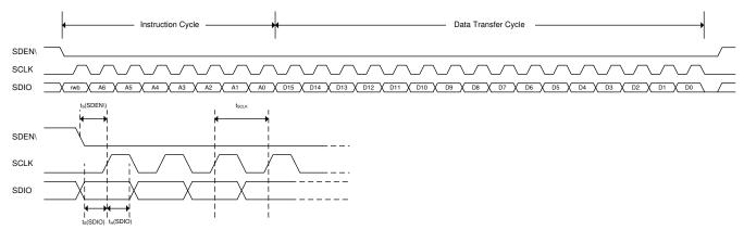
Figure 7-32. Serial Interface Write Timing Diagram
