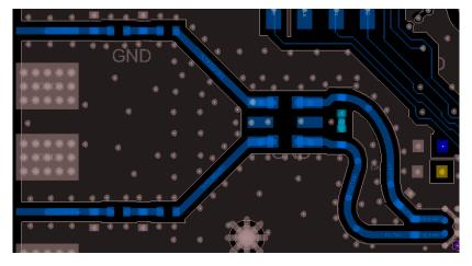
Figure 8-7. Single-ended, 50-Ω Coplanar Wave Guide RF Output Trace Example
