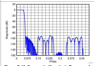
Figure 7-16. Composite Magnitude Response for 10x Interpolation
