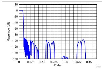
Figure 7-20. Composite Magnitude Response for 20x Interpolation
