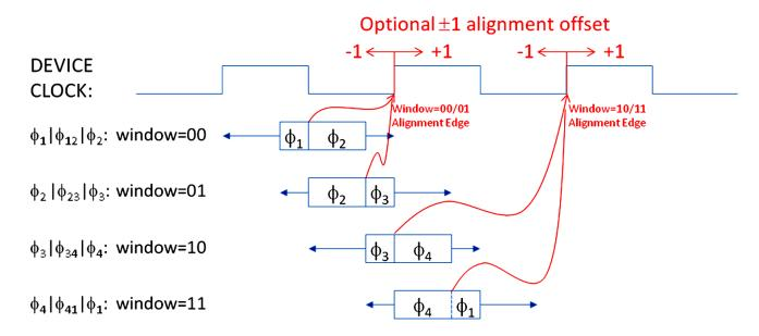
Figure 7-12. Optional SYSREF Alignment Offset
