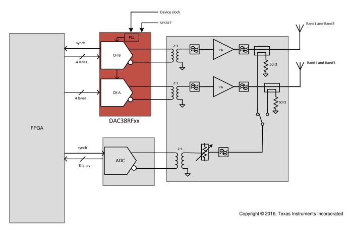
Figure 8-2. Two Antennae Multi-band Radio Frequency Transmitter
