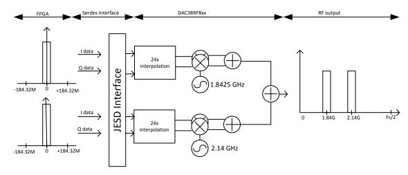
Figure 8-3. Dual Band LTE Downlink Transmitter Block Diagram
