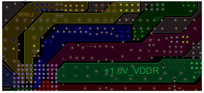
Figure 8-8. Example Power Plane Routing
