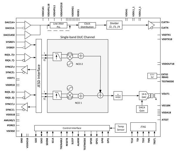
Figure 7-3. DAC38RF84 Block Diagram
