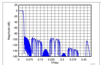
Figure 7-18. Composite Magnitude Response for 16x Interpolation
