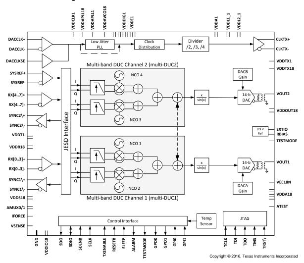
Figure 7-1. DAC38RF80 Block Diagram
