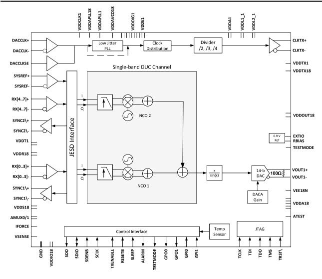
Figure 7-4. DAC38RF85 Block Diagram
