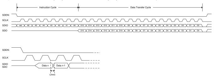
Figure 7-33. Serial Interface Read Timing Diagram
