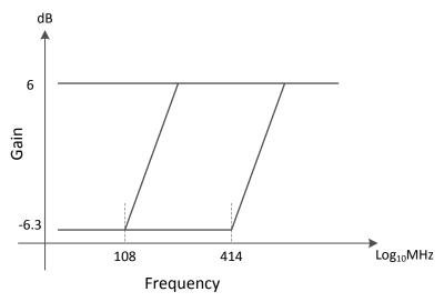
Figure 7-9. Equalizer Frequency Response
