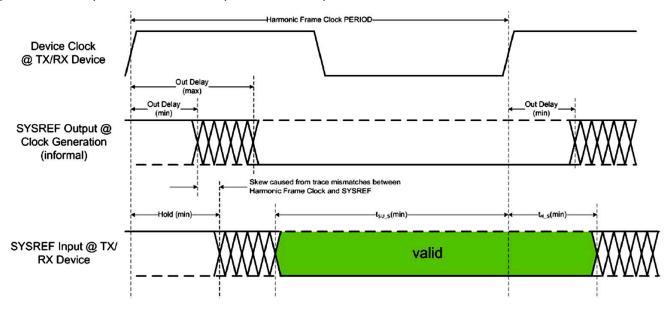
Figure 7-10. SYSREF Signal Timing
