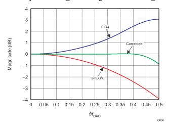
Figure 7-23. Composite Magnitude Spectrum for INVSINC
