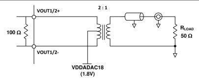
Figure 7-28. Driving a 50-Ω Load Using a 2:1 Impedance Ratio Transformer (DAC38RF83/93/85)
