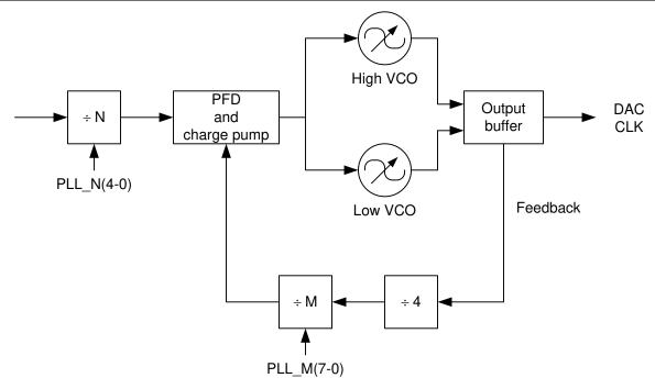
Figure 7-30. Internal PLL/VCO Block Diagram
