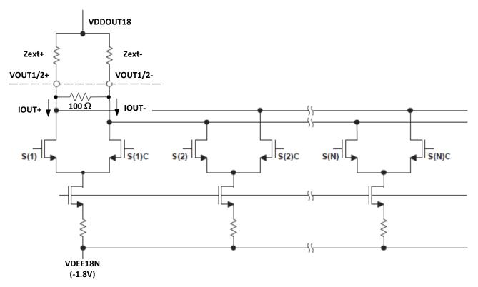
Figure 7-27. Current Steering DAC Architecture
