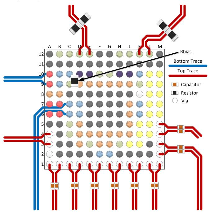
Figure 8-11. Layout Example of DAC38RFxx
