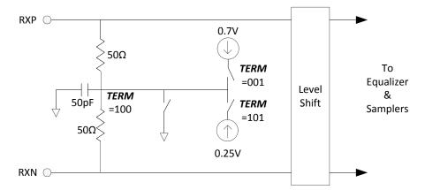
Figure 7-7. Serial Lane Input Termination
