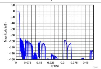
Figure 7-21. Composite Magnitude Response for 24x Interpolation
