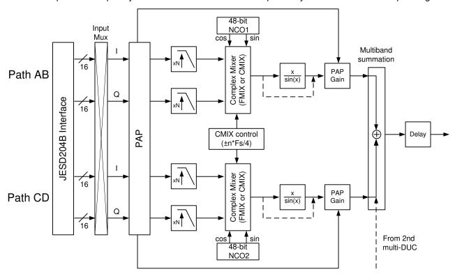
Figure 7-13. DAC38RFxx multi-DUC Signal Processing Block Diagram
