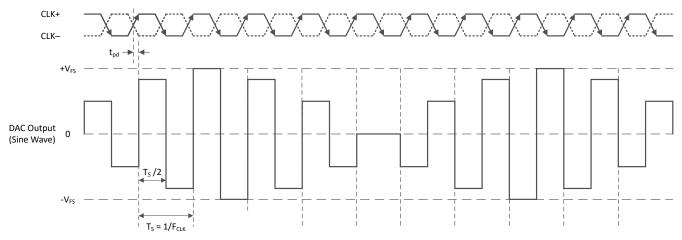
Figure 7-7. RF Mode Timing Diagram
