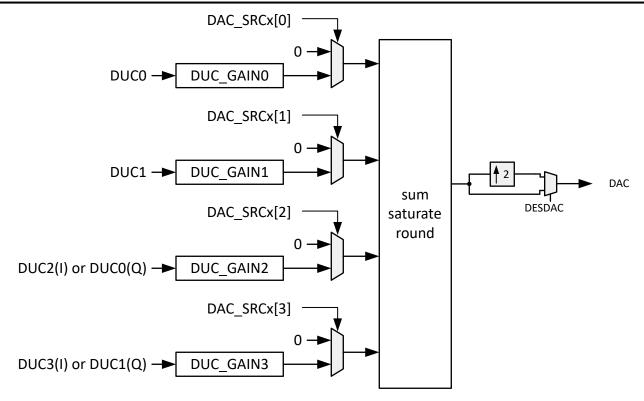
Figure 7-47. Channel Bonder Block Diagram
