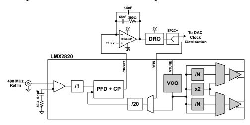
Figure 8-8. External LMX2820 with an External VCO
