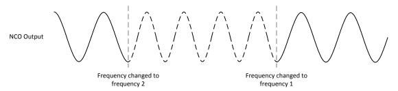
Figure 7-44. Example Phase Continuous NCO Mode Operation
