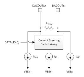
Figure 7-11. Analog Output Structure
