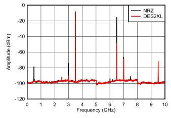
Figure 8-3. Output Spectra Comparing DES2XL and NRZ Modes
