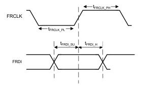
Figure 6-6. FRDI Timing Diagram
