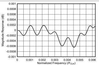
Figure 7-35. 64x Interpolation Filter Passband Response
