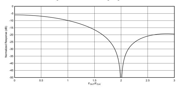
Figure 7-6. RTZ Mode Output Frequency Response
