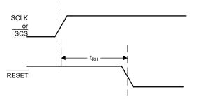
Figure 6-5. RESET Timing Diagram
