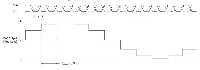
Figure 7-3. NRZ Mode Timing Diagram
