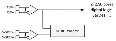
Figure 7-12. Device Clocking Subsystem
