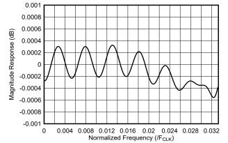
Figure 7-24. 12x Interpolation Filter Response
