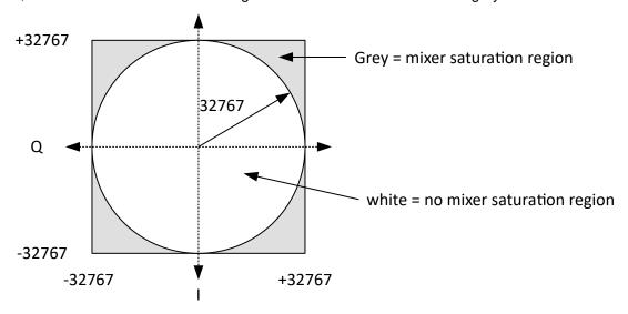
Figure 7-46. Mixer Saturation Region for the 16-bit Complex Input
