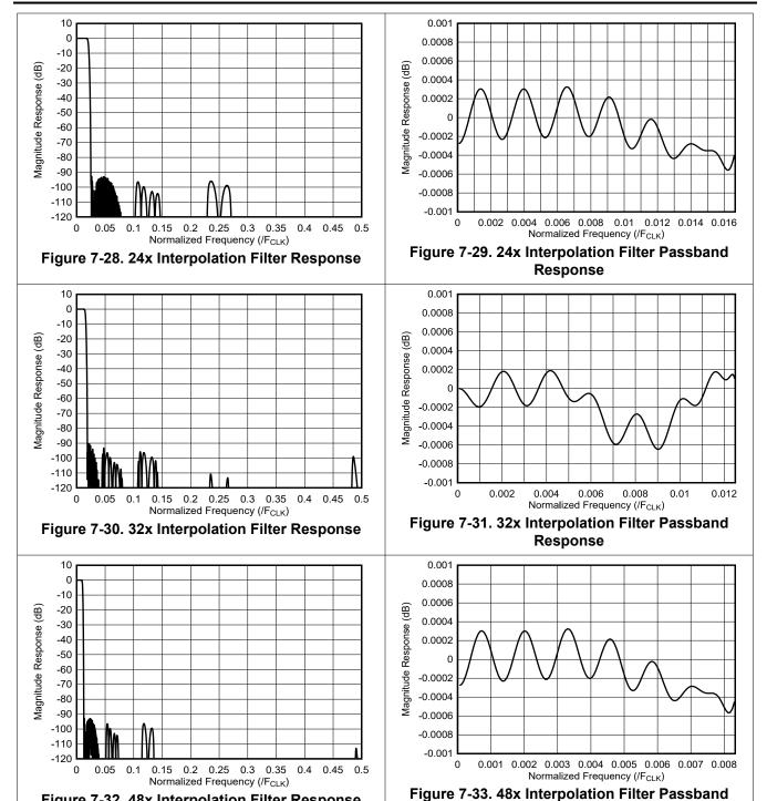
Figure 7-32. 48x Interpolation Filter Response
