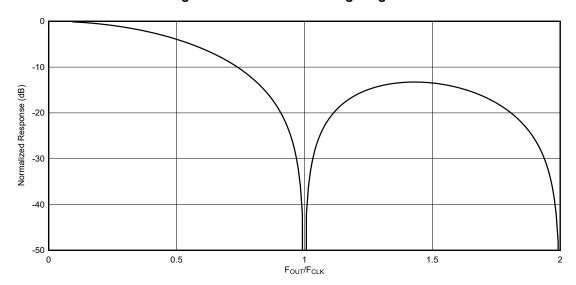
Figure 7-4. NRZ Mode Output Frequency Response
