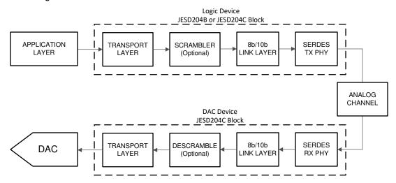
Figure 7-50. Simplified JESD204C Interface Diagram with 8b/10b Encoding
