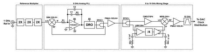
Figure 8-11. 10 GHz Clock Synthesizer
