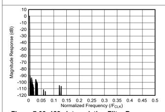
Figure 7-38. 128x Interpolation Filter Response
