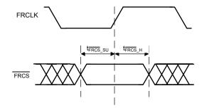
Figure 6-7. FRCS Timing Diagram
