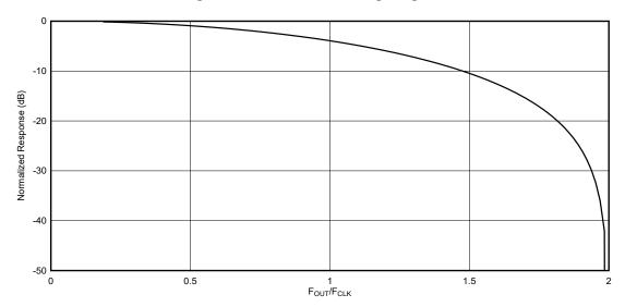
Figure 7-10. DES1X Output Frequency Response
