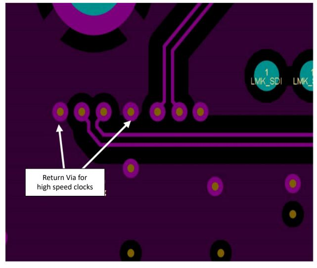
Figure 8-26. Return Vias for High Speed Clock
