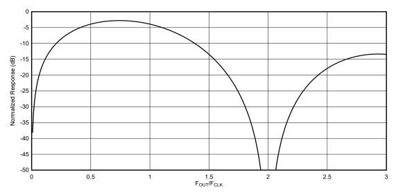
Figure 7-8. RF Mode Output Frequency Response
