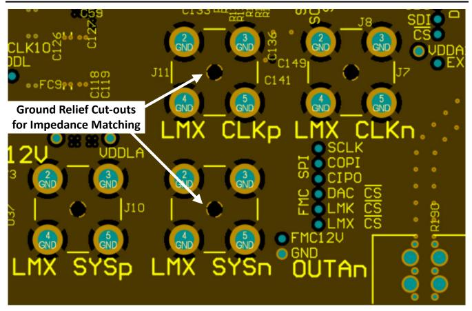
Figure 8-25. Ground Cut-out Below SMA Connector Center Pin
