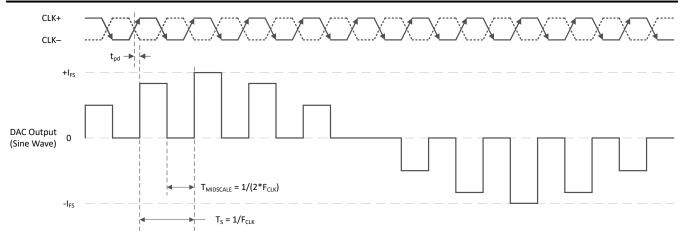
Figure 7-5. RTZ Mode Timing Diagram
