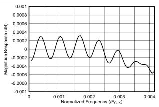
Figure 7-37. 96x Interpolation Filter Passband Response
