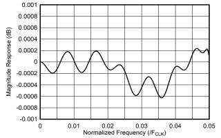
Figure 7-22. 8x Interpolation Filter Response
