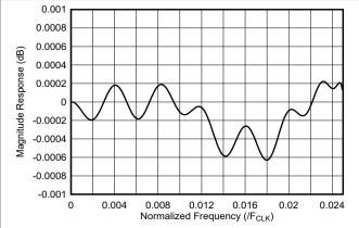
Figure 7-26. 16x Interpolation Filter Response
