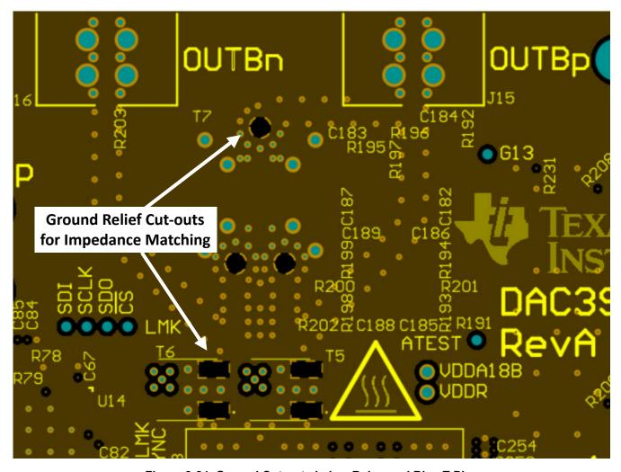
Figure 8-24. Ground Cut-outs below Balun and Bias-T Pins
