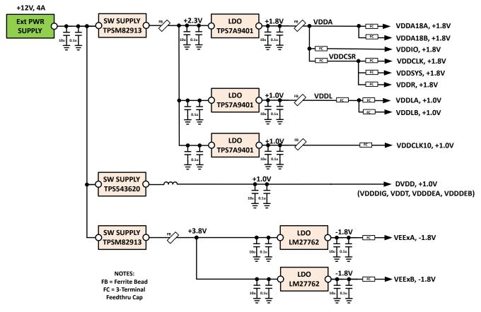
Figure 8-22. Recommended Power Supply Block Diagram
