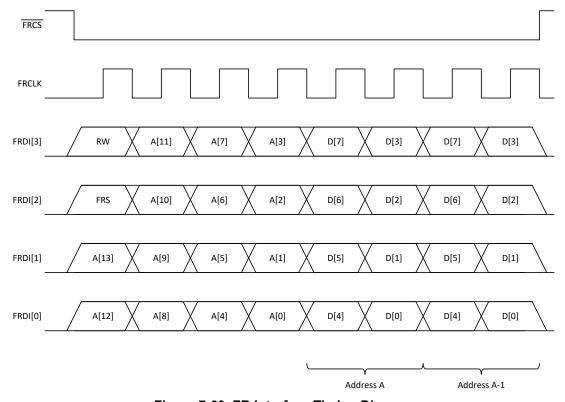
Figure 7-60. FR Interface Timing Diagram
