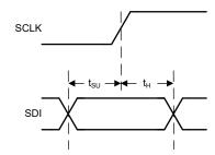
Figure 6-2. SPI Data Input Timing Diagram
