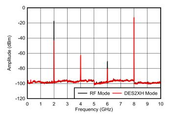
Figure 8-4. Output Spectra Comparing DES2XH and RF Modes
