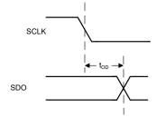
Figure 6-3. SPI Data Output Timing Diagram
