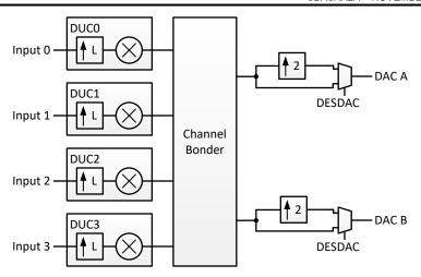
Figure 7-13. DUC Block with real output
