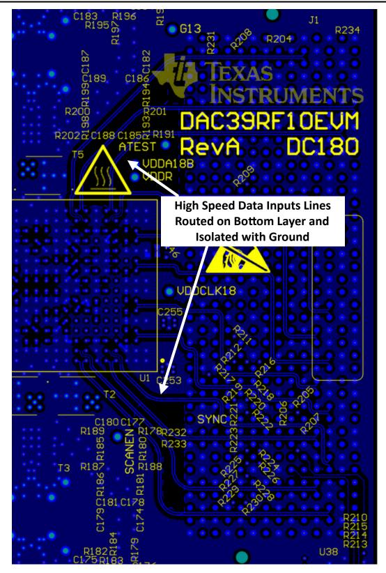
Figure 8-29. Serdes Bottom Layer Routing with Ground Isolation
