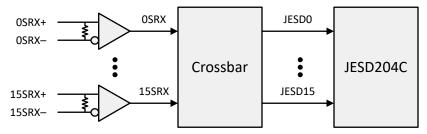
Figure 7-53. Crossbar Block Diagram
