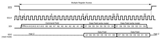
Figure 7-59. Serial Interface Protocol: Streaming Read and Write
