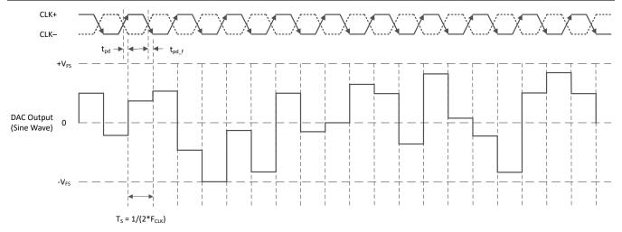
Figure 7-9. DES Mode Timing Diagram
