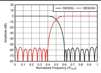
Figure 8-1. DES Interpolator Frequency Response
