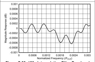
Figure 7-39. 128x Interpolation Filter Passband Response
