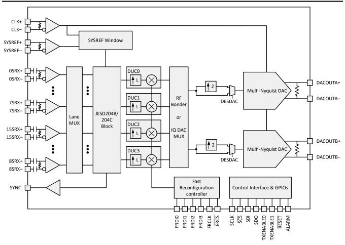
**Block Diagram (Dual Channel Devices)**
