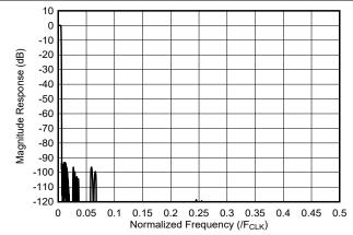
Figure 7-36. 96x Interpolation Filter Response
