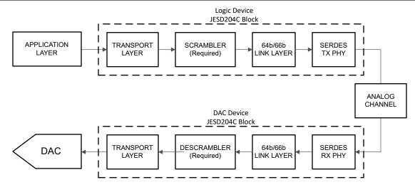
Figure 7-51. Simplified JESD204C Interface Diagram with 64b/66b Encoding
