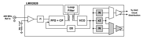
Figure 8-7. LMX2820 with Internal VCO
