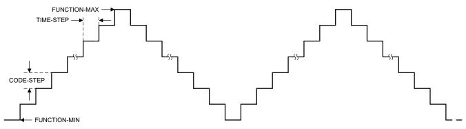
Figure 7-12. Triangle Waveform
