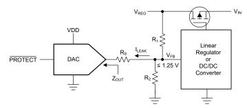
Figure 7-9. High-Impedance (Hi-Z) Output and PROTECT Input
