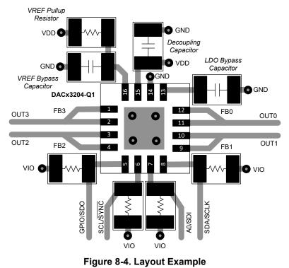
Note: The ground and power planes have been omitted for clarity. Connect the thermal pad to ground.
