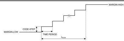
Figure 7-10. Programmable Slew-Rate Control
