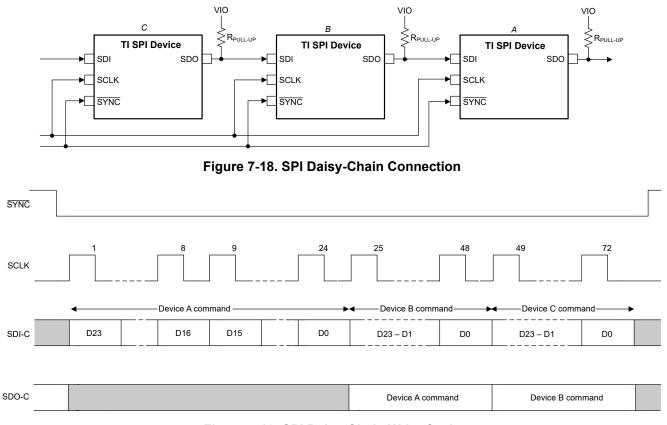
Figure 7-19. SPI Daisy-Chain Write Cycle
