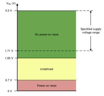
Figure 7-15. Threshold Levels for  $V_{\text{DD}}$  POR Circuit
