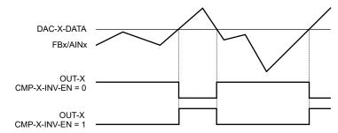
Figure 7-4. Programmable Comparator Operation
