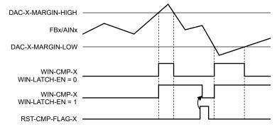
Figure 7-8. Window Comparator Operation
