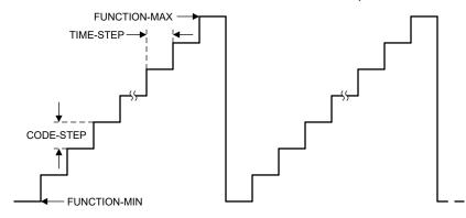
Figure 7-13. Sawtooth Waveform
