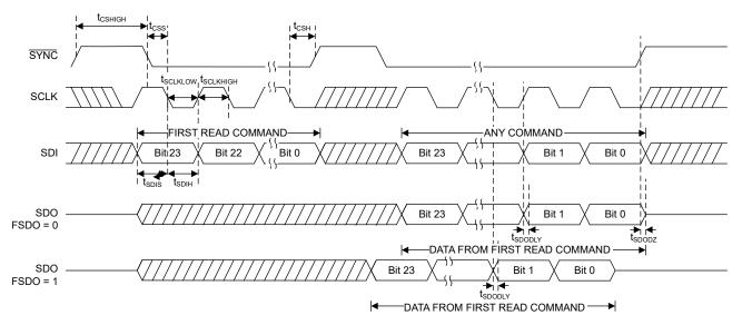
Figure 6-3. SPI Read Timing Diagram
