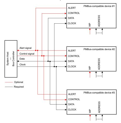
Figure 7-11. PMBus Connections
