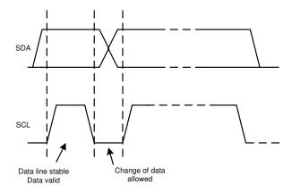
Figure 8-5. Bit Transfer on the I<sup>2</sup>C Bus
