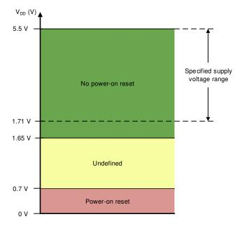
Figure 8-1. Threshold Levels for V<sub>DD</sub> POR Circuit
