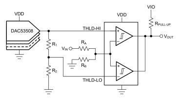
Figure 9-3. Programmable Window Comparator
