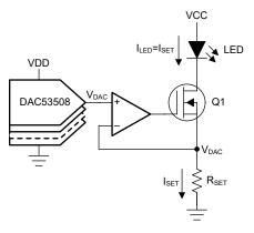
Figure 9-1. Programmable LED Biasing
