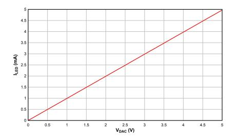
Figure 9-2. DC Transfer Characteristics of LED Biasing Circuit
