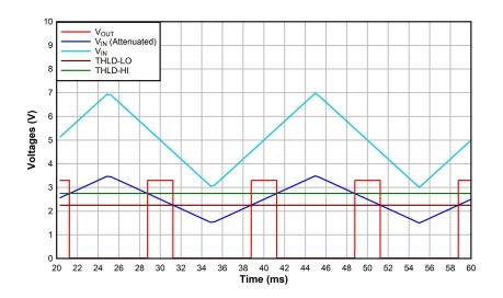
Figure 9-4. Programmable Comparator Output Waveform
