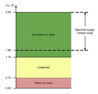
Figure 8-2. Threshold Levels for V<sub>DD</sub> POR Circuit
