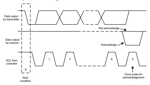
Figure 7-13. Acknowledge and Not Acknowledge on the I<sup>2</sup>C Bus
