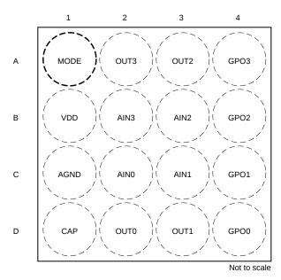
Figure 5-1. YBH Package, 16-pin DSBGA (Top View)
