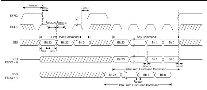
Figure 6-3. SPI Read Timing Diagram
