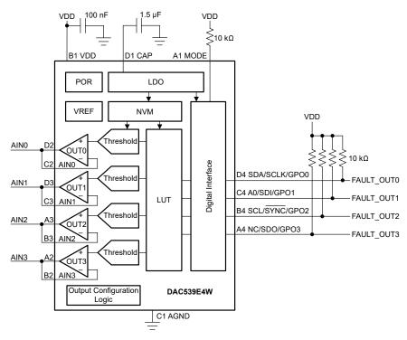
Figure 8-1. LUT-Based Standalone Fault-Management Circuit
