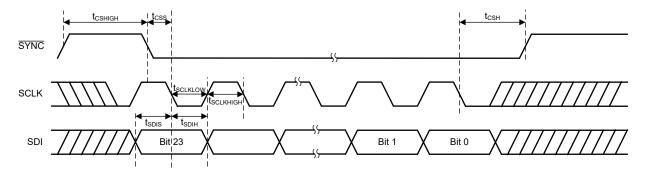
Figure 6-2. SPI Write Timing Diagram
