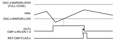
Figure 7-8. Latching Comparator With Active-High Output
