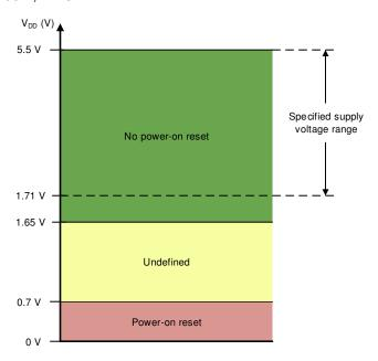
Figure 7-3. Threshold Levels for V<sub>DD</sub> POR Circuit
