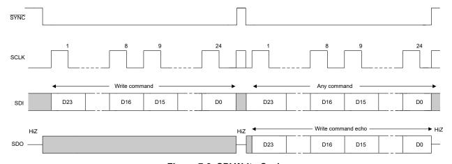
Figure 7-9. SPI Write Cycle
