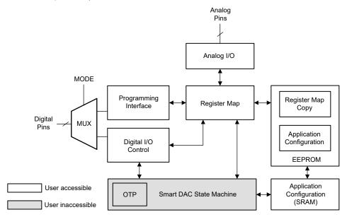
Figure 7-1. Smart DAC Architecture
