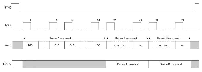
Figure 7-12. SPI Daisy-Chain Write Cycle
