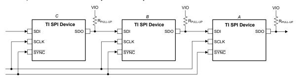
Figure 7-11. SPI Daisy-Chain Connection
