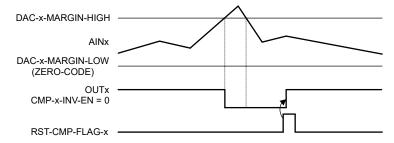
Figure 7-7. Latching Comparator With Active-Low Output
