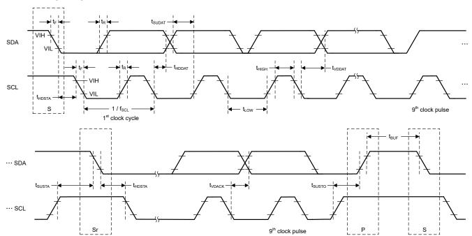
S: Start bit, Sr: Repeated start bit, P: Stop bit
