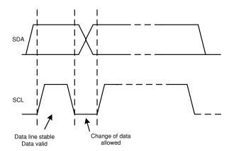
Figure 7-15. Bit Transfer on the I<sup>2</sup>C Bus
