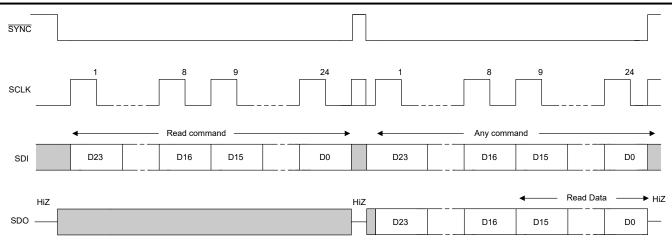
Figure 7-10. SPI Read Cycle
