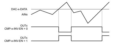
Figure 7-5. Programmable Comparator Operation
