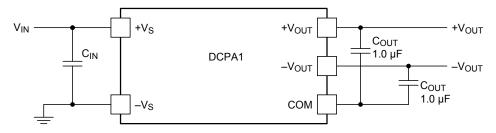
Figure 35. Dual Output Devices Connected in Series
