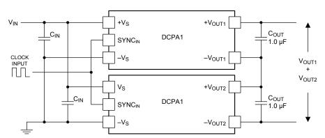
Figure 34. Multiple DCPA1 Devices Connected in Series
