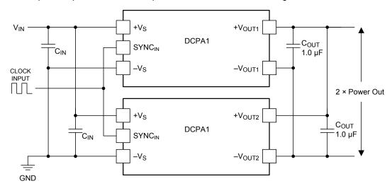
Figure 36. Multiple DCPA1 Devices Connected in Parallel
