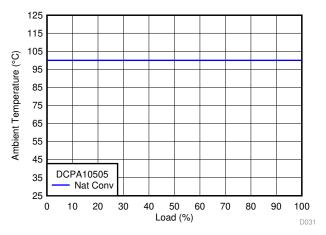
Figure 33. Thermal Safe Operating Area
