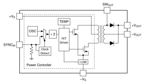
Figure 31. Single Output Device
