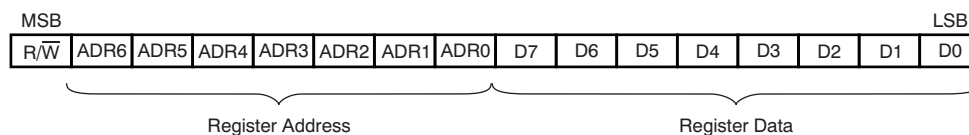
Figure 19. Control Data Word Format for MDI
