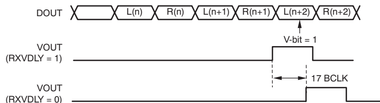
Figure 8. RXVDLY and VOUT Timing
