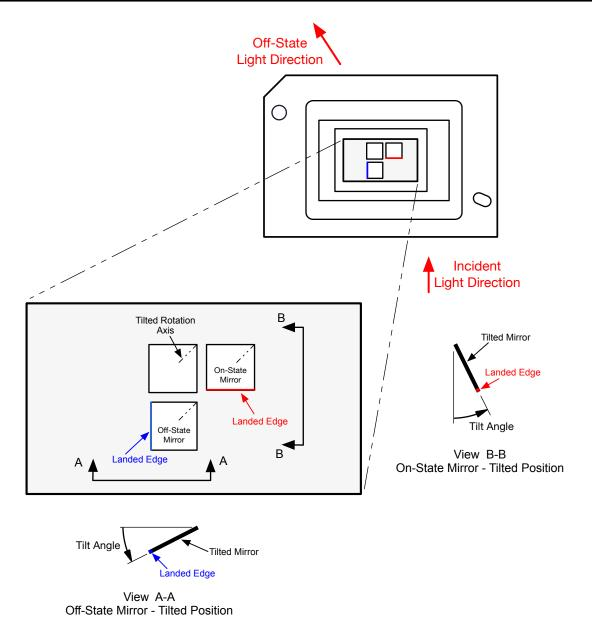
Figure 6-10. Micromirror Landed Orientation and Tilt
