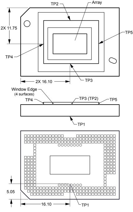
Figure 7-2. DMD Thermal Test Points
