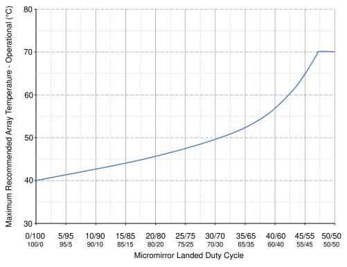
Figure 6-1. Maximum Recommended Array Temperature—Derating Curve
