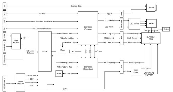
Figure 8-1. Typical DLP500YX Application Diagram
