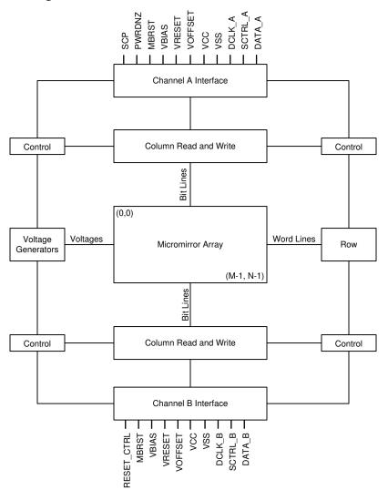
Channels C and D not shown. For pin details on channels A, B, C, and D, refer to the *Pin Configurations and Functions* table and the LVDS interface section of *Section 6.8*.
