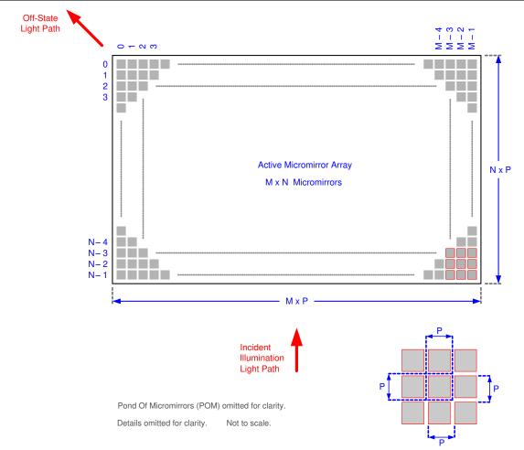
Figure 6-9. Micromirror Array Physical Characteristics
