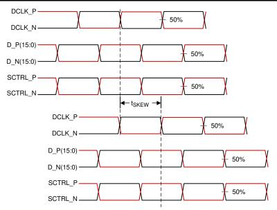
Figure 6-7. LVDS Interface Channel Skew Definition
