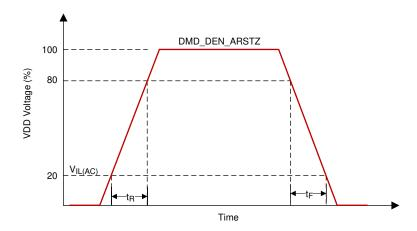
Figure 6-10. LVCMOS Rise, Fall Time Slew Rate
