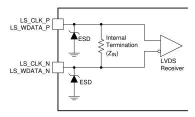
Figure 6-8. LSIF Equivalent Input
