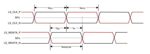
Figure 6-5. LSIF Timing Requirements
