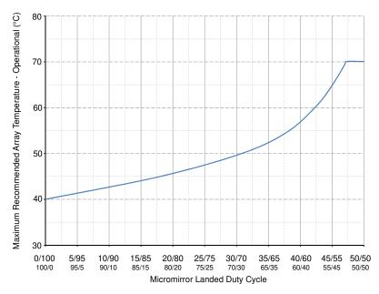
Figure 6-1. Maximum Recommended Array Temperature - Derating Curve
