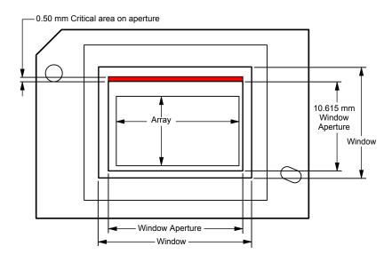
Figure 6-2. Illumination Overfill Diagram - Critical Area
