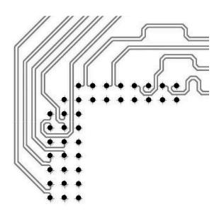
Figure 10-1. Example HSSI PCB Routing
