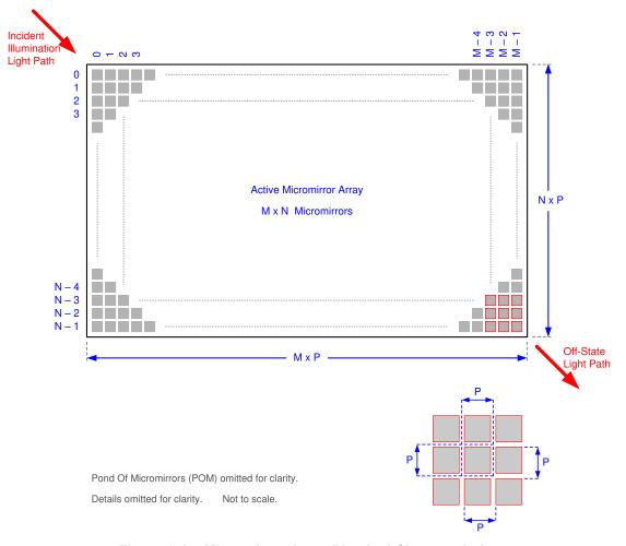
Figure 6-15. Micromirror Array Physical Characteristics
