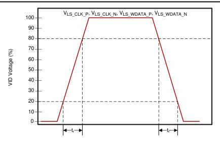
Figure 6-6. LSIF Rise, Fall Time Slew Rate
