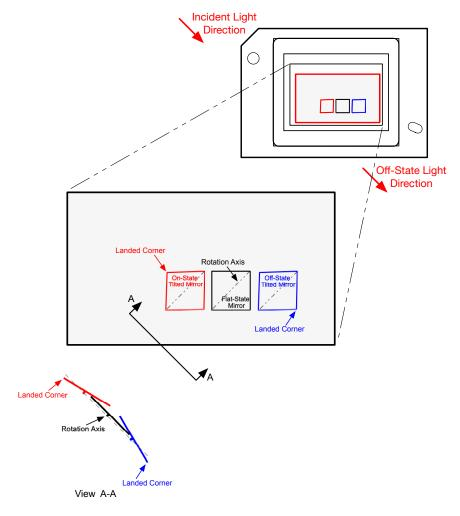
Figure 6-16. Micromirror Landed Orientation and Tilt
