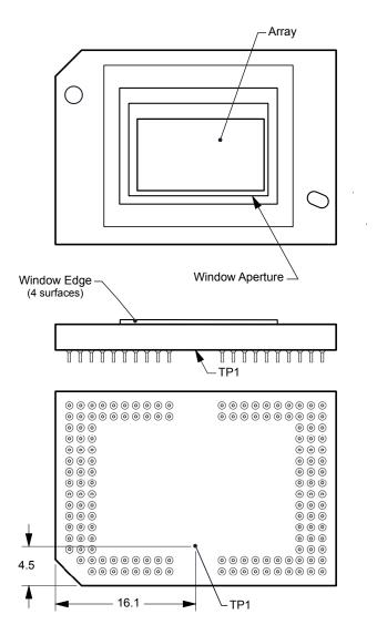
Figure 7-1. DMD Thermal Test Point
