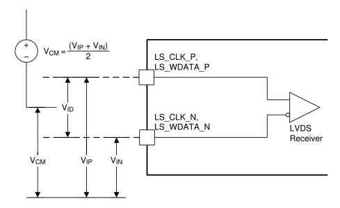
Figure 6-7. LSIF Voltage Requirements
