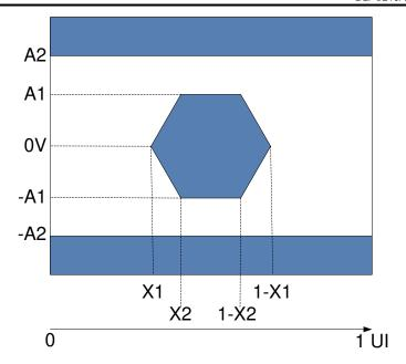
Figure 6-12. HSSI Eye Characteristics
