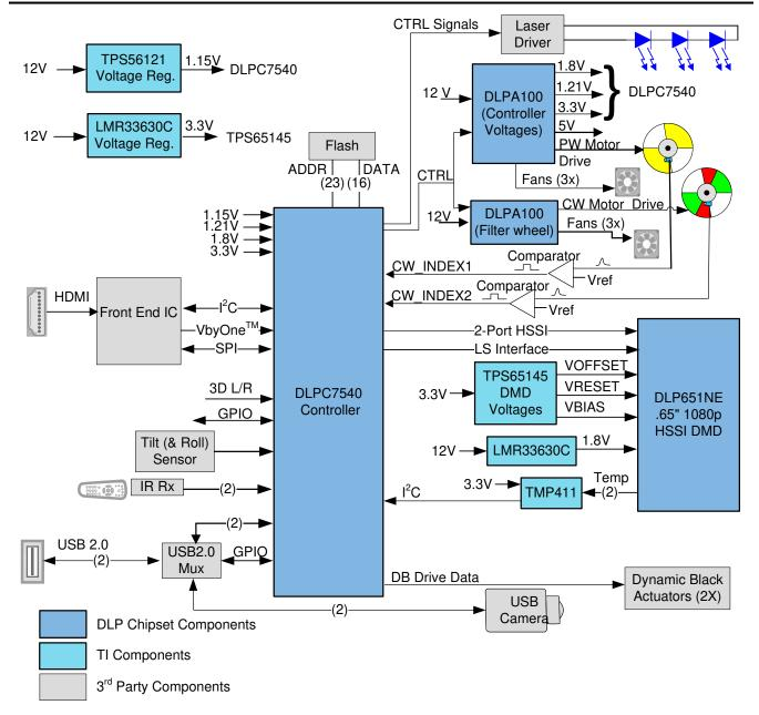
Figure 8-1. Typical 1080p Laser Phosphor Application Diagram
