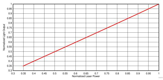
Figure 8-3. Normalized Light Output vs Normalized Laser Power for Laser Phosphor Illumination
