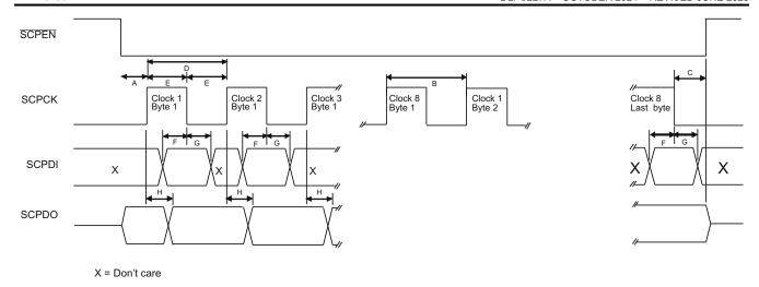
Figure 6-1. Serial Interface Timing
