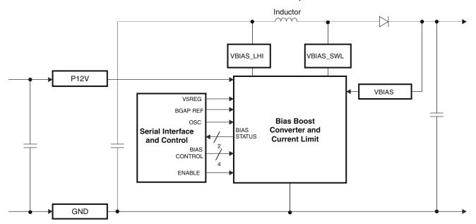
Figure 7-2. Bias Voltage Boost Converter Block Diagram
