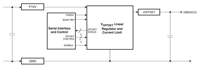
Figure 7-3. Offset Voltage Boost Convertor Block Diagram
