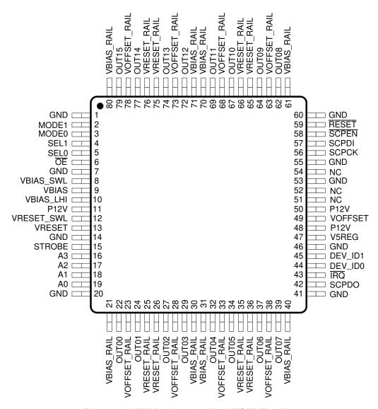
Figure 5-1. PFP Package 80-Pin HTQFP Top View
