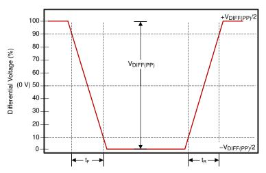
$V_{\text{CM}}$  is removed when signals are viewed differentially
