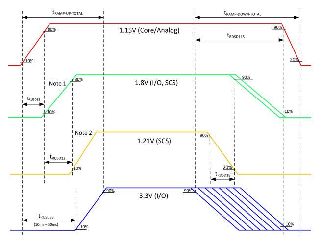
Note 1: No power up or power down timing dependency between 1.8V and 3.3V Note 2: No power up or power down timing dependency between 1.21V and 3.3V
