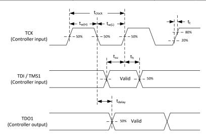
Figure 6-19. Timing Diagram for JTAG Boundary Scan
