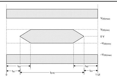
Figure 6-10. HSSI Eye Characteristics
