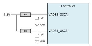
Figure 10-11. Crystal Power Supply Filtering
