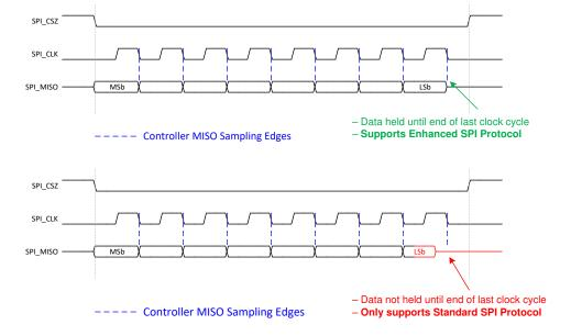
Figure 6-17. Requirement for Enhanced SPI Protocol
