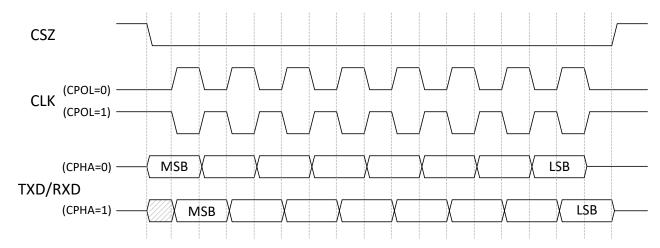
Figure 6-16. Timing Diagram for SPI Clocking Modes
