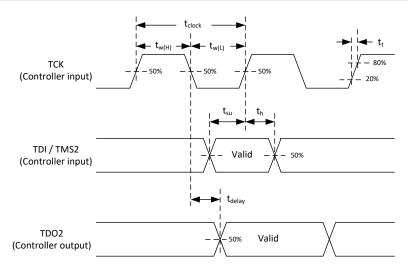
Figure 6-20. Timing Diagram for JTAG ARM Multi-Ice
