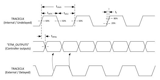
Figure 6-21. Timing Diagram for Multi-Trace ETM
