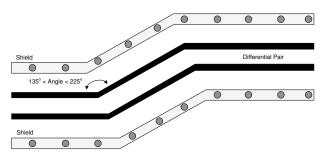
Figure 10-13. FPD-Link Routing Example
