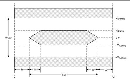
Figure 6-14. FPD-Link Timing
