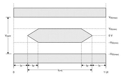
Figure 6-12. V-by-One Timing
