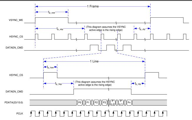
Figure 6-15. Source Frame Timing
