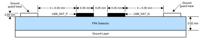
Figure 10-14. USB Layout Example
