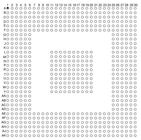
Figure 5-1. ZDC Package 676-Pin PBGA Top View
