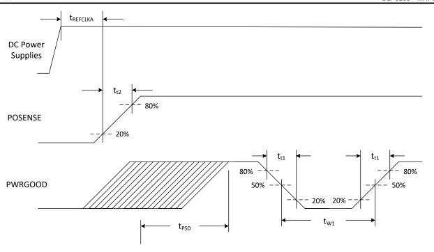
Figure 6-7. Power Up Timing
