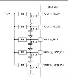
Figure 10-7. 1.15-V PLL Power Supply Filter Topology
