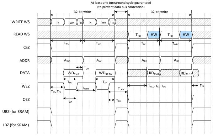
Figure 7-4. Program Memory Interface Timing Diagram
