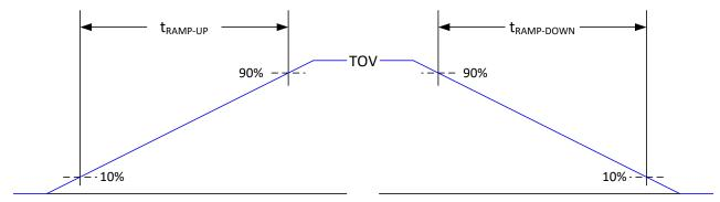
Figure 6-5. Power Supply Ramp Time
