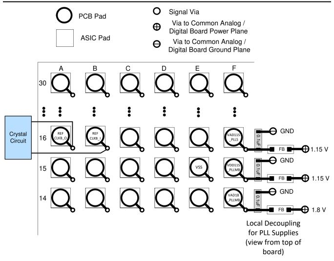
Figure 10-9. PLL Power Supply Filter Layout Examples
