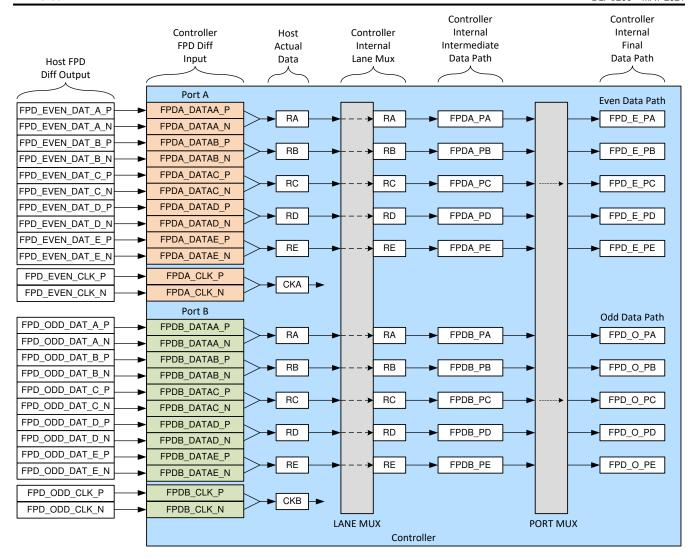
Figure 7-2. Example of Typical FPD-Link Port Lane Mapping
