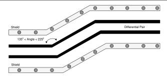
Figure 10-15. USB Routing Example
