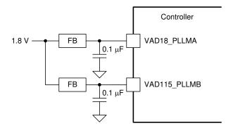
Figure 10-8. 1.8-V PLL Power Supply Filter Topology
