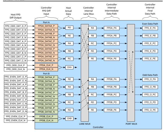
Figure 7-3. Example of Alternate FPD-Link Port Lane Mapping
