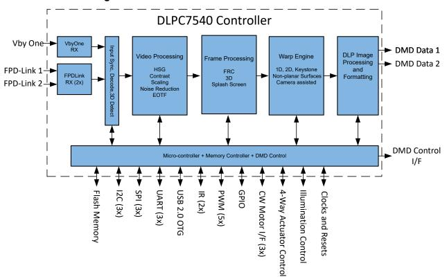
Figure 7-1. Functional Block Diagram
