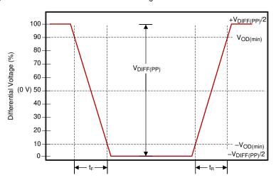
$V_{\text{CM}}$  is removed when signals are viewed differentially
