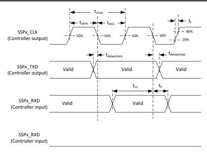
Figure 6-18. Timing Diagram for SSP Master (Modes 0/3)
