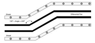
Figure 10-12. V-by-One Routing Example
