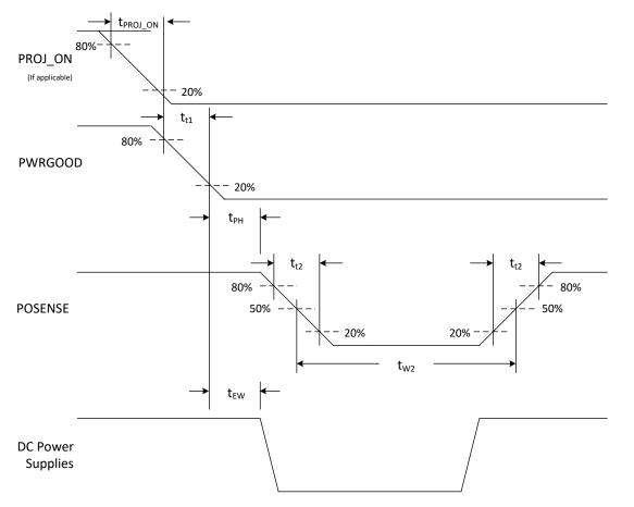
Figure 6-8. Power Down Timing
