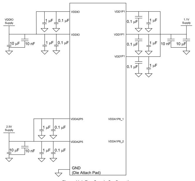
Figure 11-1. Two-Supply Configuration
