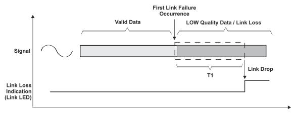
Figure 9-5. Fast Link Drop Mechanism
