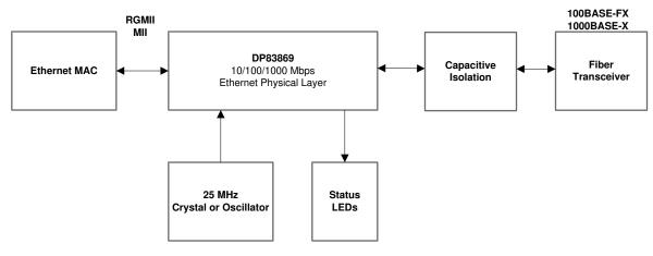
Figure 10-4. Typical Fiber Ethernet Application
