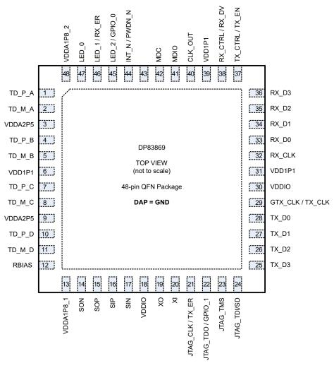
Figure 7-1. RGZ Package (48-Pin VQFN) Top View
