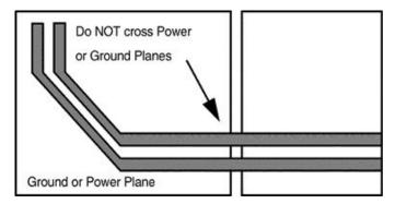
Figure 12-2. Differential Signal Pair-Plane Crossing
