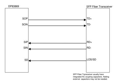
Figure 10-5. PHY to Fiber Transceiver Connections
