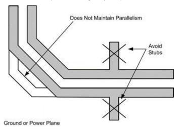
Figure 12-1. Avoiding Stubs in a Differential Signal Pair
