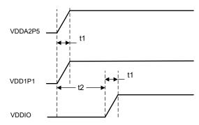
Figure 11-2. Two-Supply Sequence Diagram
