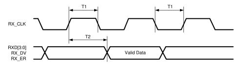
Figure 8-5. 100-Mbps MII Receive Timing
