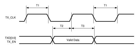
Figure 8-4. 100-Mbps MII Transmit Timing
