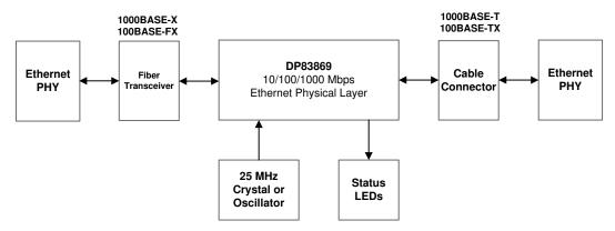
Figure 5-1. Media Convertor System Block Diagram
