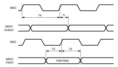
Figure 8-8. Serial Management Interface Timing
