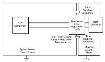
Figure 12-5. Copper Ethernet Layout Example
