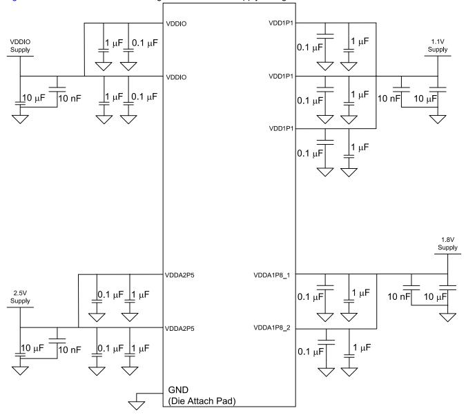
Figure 11-3. Three-Supply Configuration
