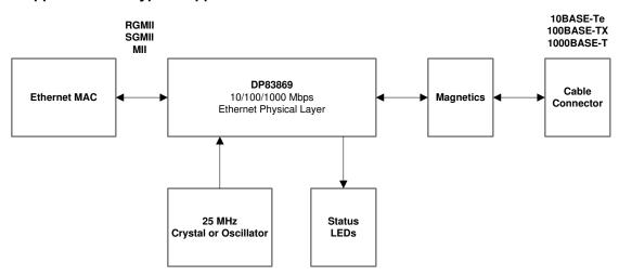
Figure 10-1. Typical Copper Ethernet Application
