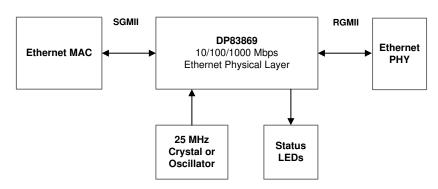
Figure 5-3. SGMII-RGMII Bridge System Block Diagram
