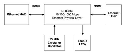
Figure 5-2. RGMII-SGMII Bridge System Block Diagram
