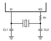
Figure 10-2. Crystal Oscillator Circuit
