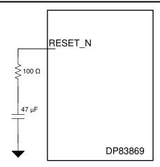
Figure 9-17. RESET\_N Circuit
