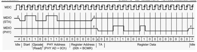
Figure 9-13. Typical MDC/MDIO Read Operation
