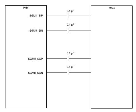
Figure 9-6. SGMII 4-Wire Connections
