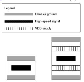
Figure 12-4. Alternative Layer Stack-Up
