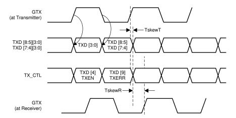
Figure 8-6. RGMII Transmit Multiplexing and Timing Diagram
