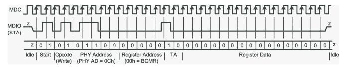
Figure 9-14. Typical MDC/MDIO Write Operation
