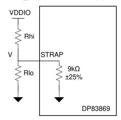
Figure 9-15. Strap Circuit
