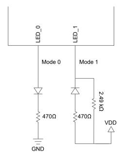
Figure 9-16. Example Strap Connections
