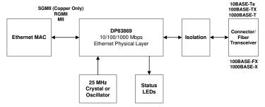
Standard Ethernet System Block Diagram
