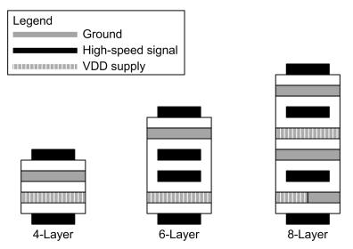
Figure 12-3. Recommended Layer Stack-Up
