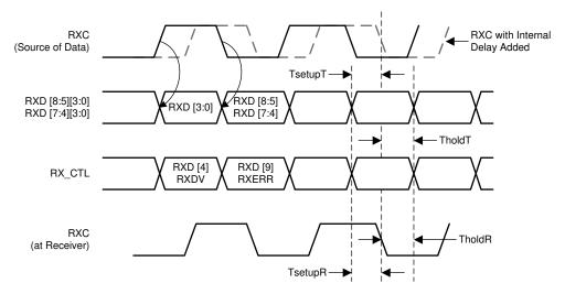
Figure 8-7. RGMII Receive Multiplexing and Timing Diagram
