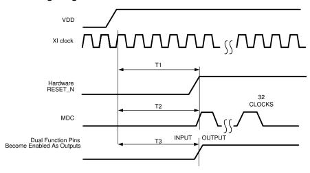
Figure 8-1. Power-Up Timing
