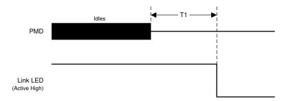
Figure 8-3. Copper Link Timing
