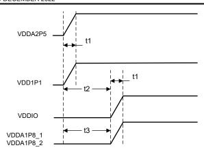
Figure 11-4. Three-Supply Sequence Diagram
