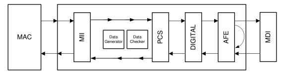
Figure 7-4. Analog Loopback With External Data-Gen
