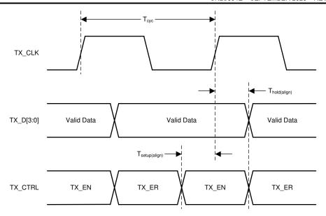
Figure 6-4. RGMII Transmit Timing (Internal Delay Disabled)
