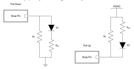
Figure 7-19. Example Strap Connections
