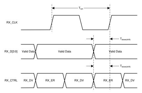
Figure 6-5. RGMII Receive Timing (Internal Delay Enabled)
