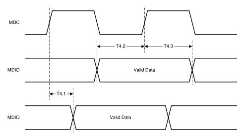
Figure 6-7. Serial Management Timing
