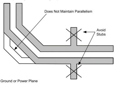
Figure 11-1. Differential Signal Trace Routing
