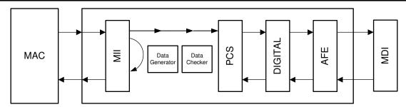
Figure 7-9. xMII Loopback With External Data-Gen
