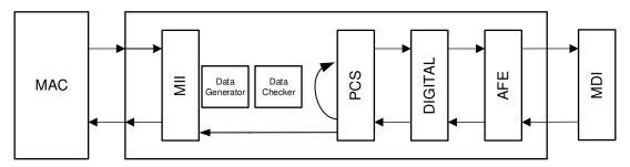
Figure 7-10. xMII Reverse Loopback With External Data-Gen
