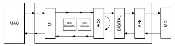
Figure 7-8. PCS Loopback With External Data-Gen
