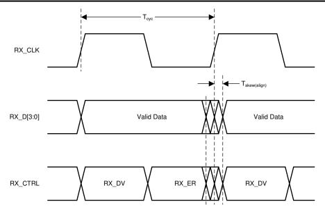
Figure 6-6. RGMII Receive Timing (Internal Delay Disabled)
