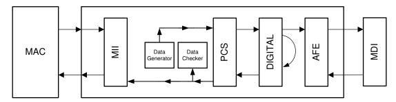
Figure 7-5. Digital Loopback With Inbuilt Data-Gen
