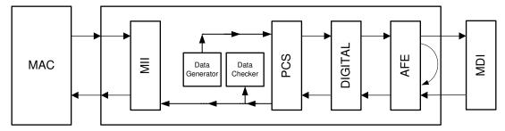
Figure 7-3. Analog Loopback With Inbuilt Data-Gen
