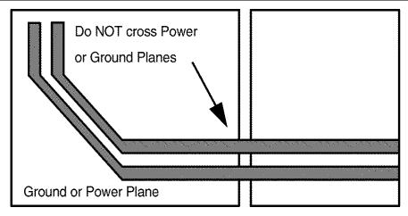
Figure 11-2. Power and Ground Plane Breaks
