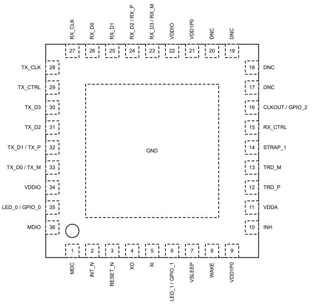
Figure 5-1. RHA Package 36-Pin VQFN **Top View**
