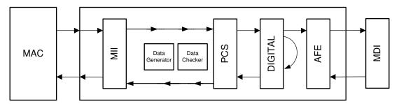
Figure 7-6. Digital Loopback With External Data-Gen
