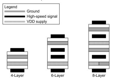
Figure 11-3. Recommended PCB Layer Stack-Up
