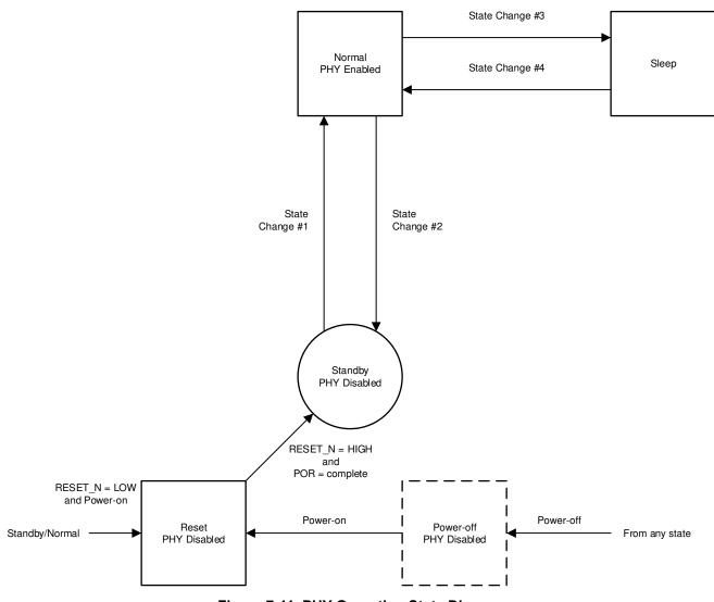
Figure 7-11. PHY Operation State Diagram
