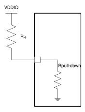
Figure 7-18. Strap Circuit
