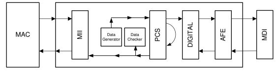
Figure 7-7. PCS Loopback With Inbuilt Data-Gen
