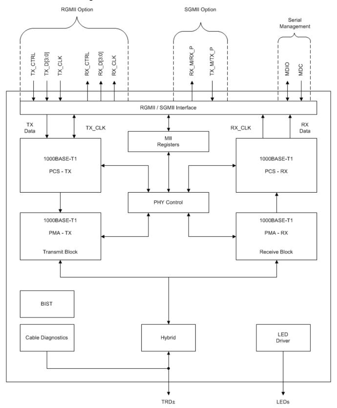
Figure 7-1. DP83TG720S-Q1 Functional Block Diagram
