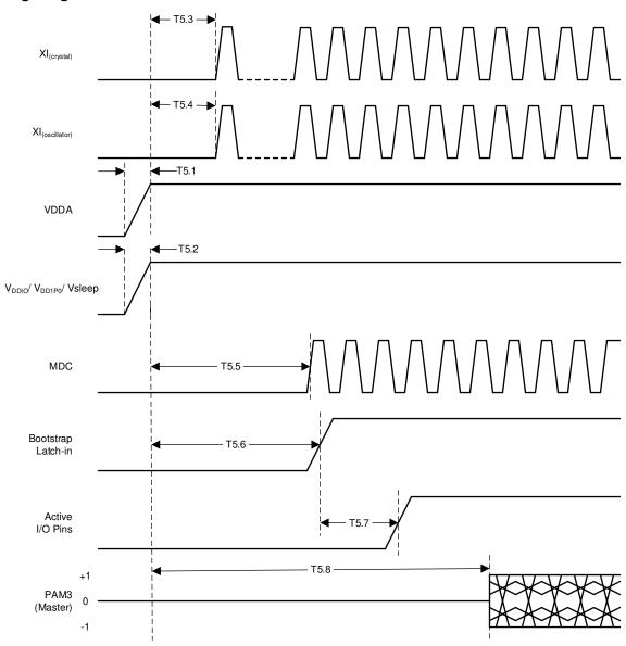
Figure 6-1. Power Up Timing
