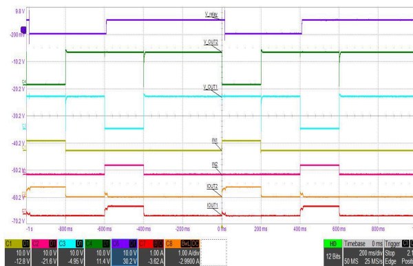
A. Ch 1 = IN1 Ch 2 = IN2 Ch 3 = V OUT1 Ch 4 = V OUT2 Ch 6 = Relay Switch Ch 7 = Relay Coil1 Current Ch 8 = Relay Coil2 Current
