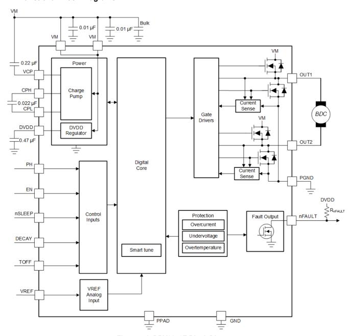
Figure 7-1. DRV8256E Block Diagram
