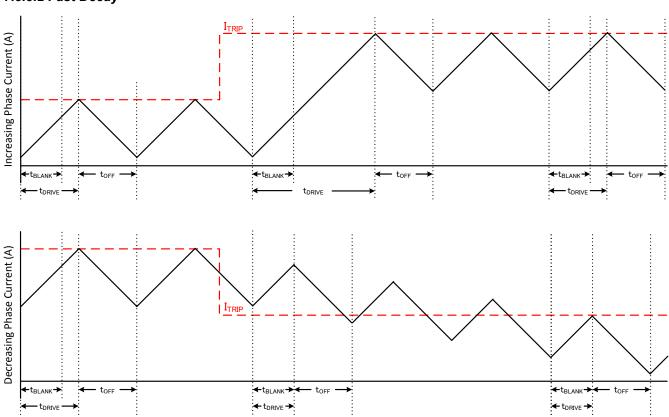
Figure 7-6. Fast/Fast Decay Mode
