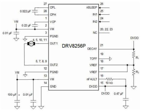
Figure 8-1. Typical Application Schematic
