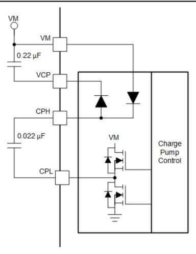
Figure 7-9. Charge Pump Block Diagram
