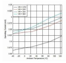
Figure 6-4. Operating Current over Temperature
