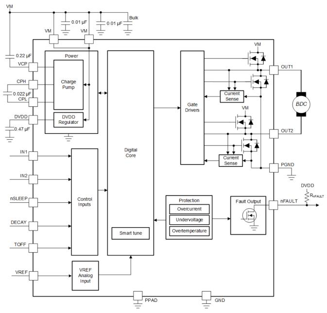
Figure 7-2. DRV8256P Block Diagram
