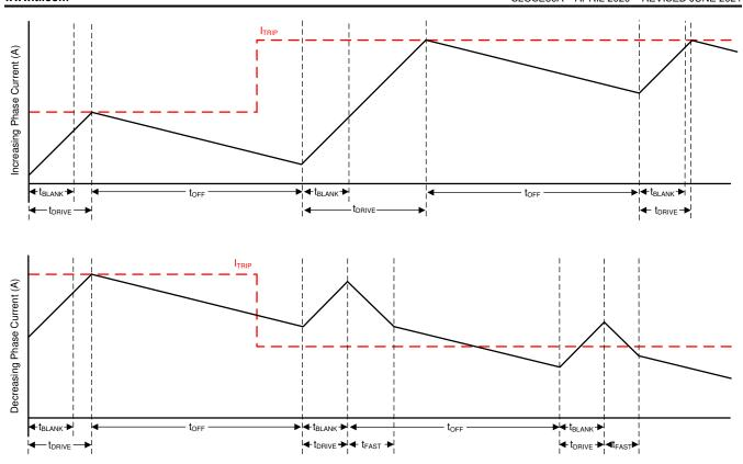
Figure 7-7. Smart tune Dynamic Decay Mode
