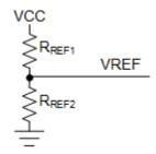
Figure 7-3. Resistor divider connected to the VREF pins
