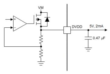
Figure 7-10. Linear Voltage Regulator Block Diagram
