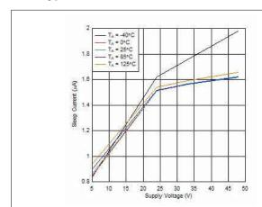
Figure 6-1. Sleep Current over Supply Voltage
