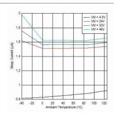
Figure 6-2. Sleep Current over Temperature
