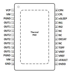
Figure 5-3. PWP PowerPAD™ Package 28-Pin HTSSOP Top View DRV8256P
