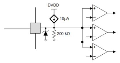
Figure 7-12. Quad-Level Input Pin Diagram
