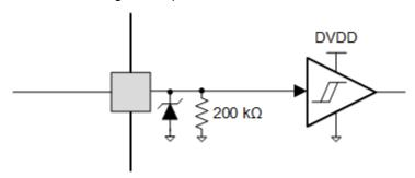
Figure 7-11. Logic-level Input Pin Diagram
