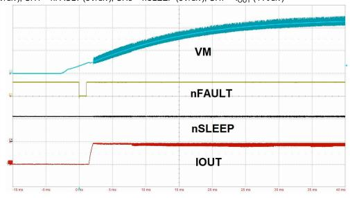
Figure 8-3. Device Power-up with Supply Voltage (VM) Ramp
