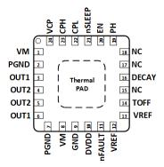
Figure 5-2. RGE Package 24-Pin VQFN with Exposed Thermal PAD Top View DRV8256E
