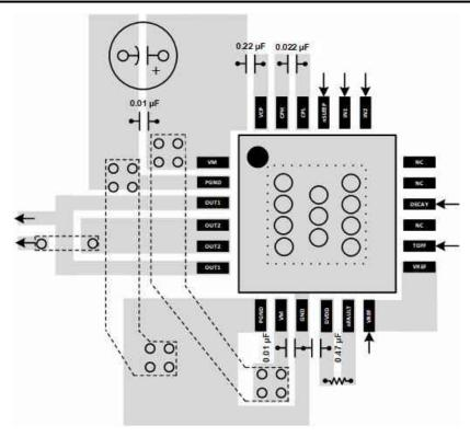
Figure 10-2. QFN Layout Example
