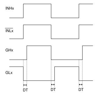
Figure 8-4. Inverted INLx inputs
