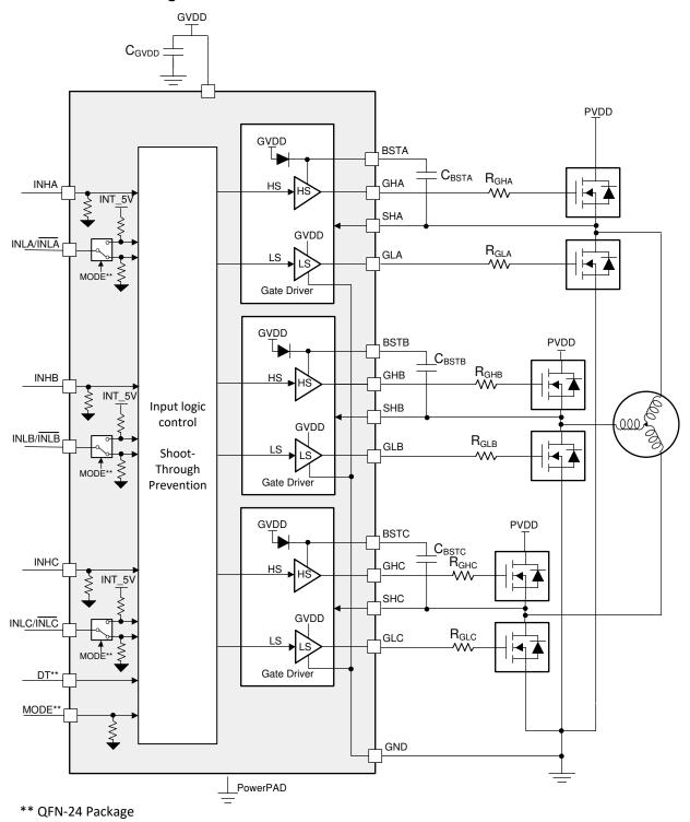
Figure 8-1. Block Diagram for DRV8300UD
