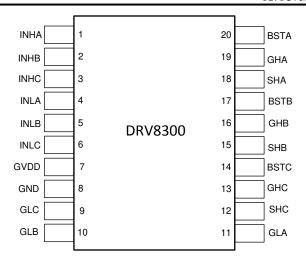
Figure 6-2. DRV8300UD, DRV8300UDI PW Package 20-Pin TSSOP Top View
