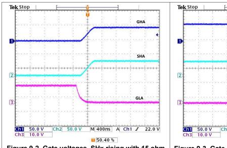
Figure 9-2. Gate voltages, SHx rising with 15 ohm gate resistor and CSD19532Q5B MOSFET
