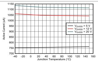
Figure 7-4. Supply Current Over Temperature
