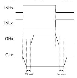
Figure 7-2. Propagation Delay Match (t<sub>PD match</sub>)
