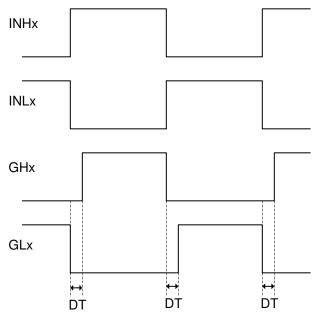
Figure 8-3. Non-Inverted INLx inputs
