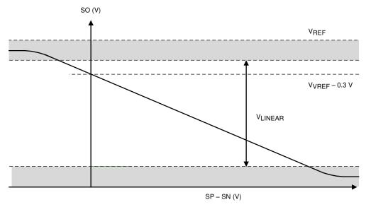
Figure 34. Unidirectional Current-Sense Output
