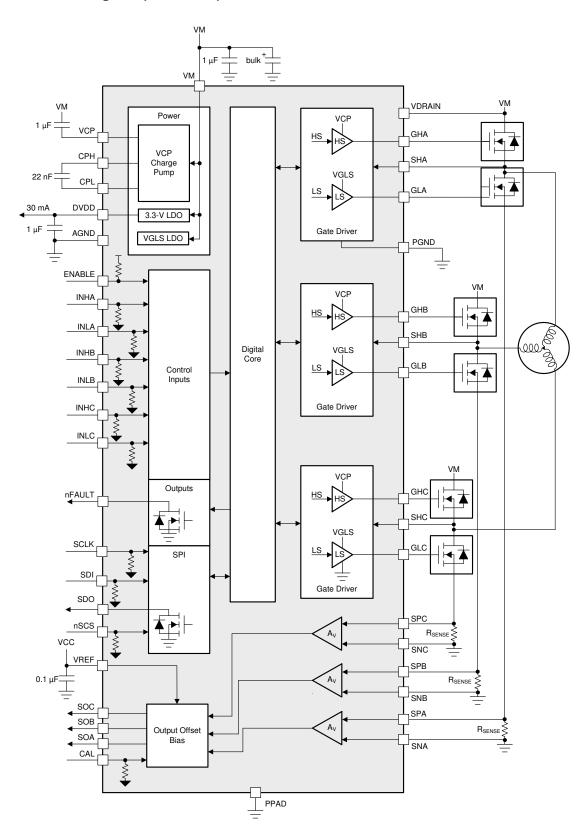
Figure 11. Block Diagram for DRV8304S
