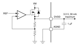
Figure 24. DVDD Linear Regulator Block Diagram
