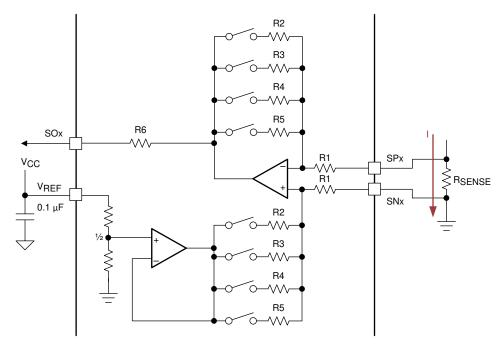
Figure 30. Bidirectional Current-Sense Configuration
