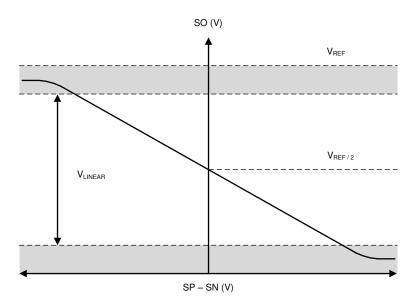
Figure 31. Bidirectional Current-Sense Output
