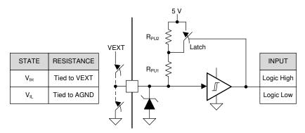
Figure 26. Logic-Level Input Pin Structure (ENABLE)
