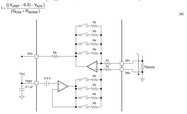
Figure 33. Unidirectional Current-Sense Configuration
