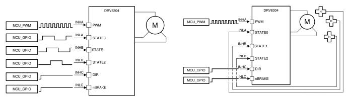
Figure 12. 1x PWM—Simple Controller
