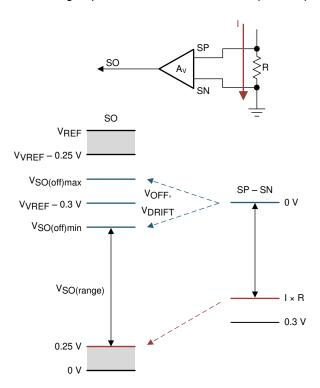
Figure 58. Sense Amplifier Configuration
