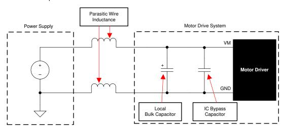
Figure 59. Motor Drive Supply Parasitics Example
