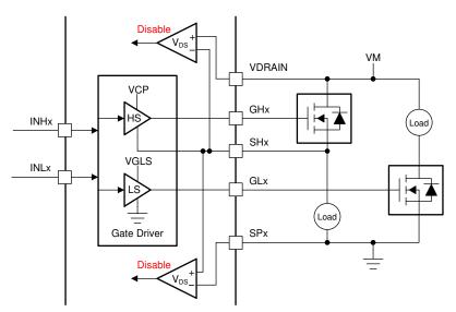
Figure 14. Independent PWM High-Side and Low-Side Drivers
