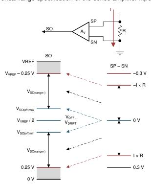
Figure 46. Sense Amplifier Configuration
