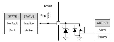
Figure 29. Open-Drain Output Pin Structure
