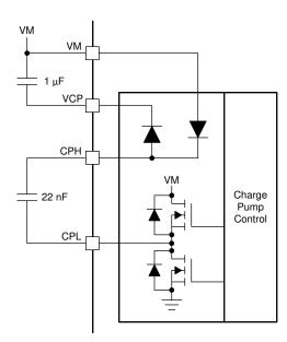
Figure 19. Charge Pump Architecture
