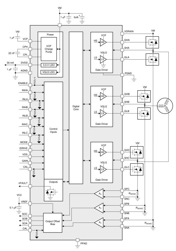
Figure 10. Block Diagram for DRV8304H
