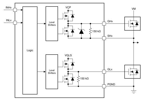
Figure 20. Gate Driver Block Diagram
