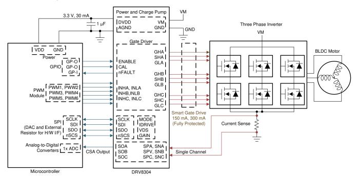
Figure 57. Alternative Application Schematic
