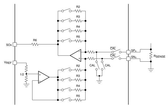
Figure 36. Amplifier Calibration Mode
