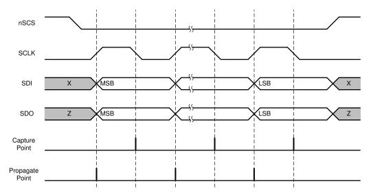
Figure 37. SPI Slave Timing Diagram
