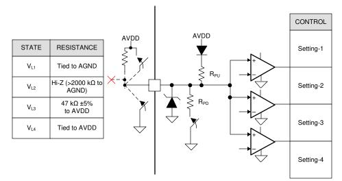
Figure 8-26. Four Level Input Pin Structure
