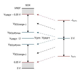
Figure 8-28. Bidirectional Current Sense Output
