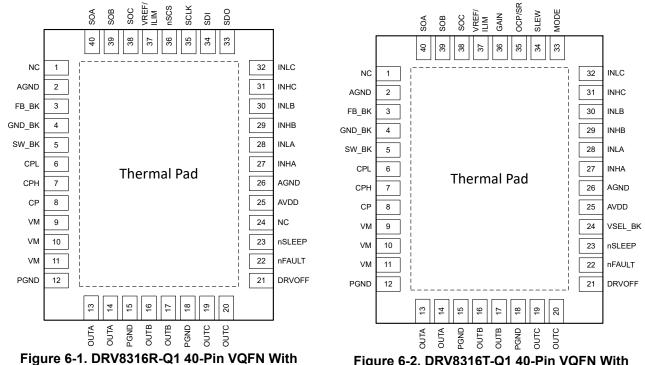
Exposed Thermal Pad Top View
