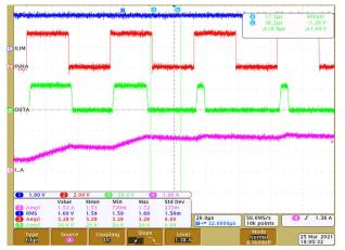
Figure 9-11. Driver PWM with Current Limit
