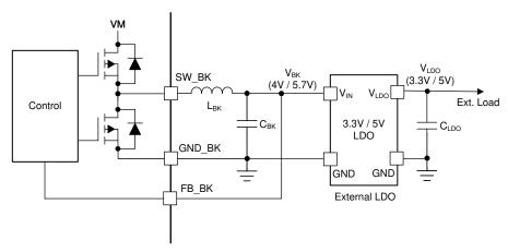
Figure 8-10. Buck Regulator with External LDO
