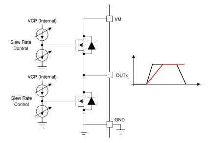
Figure 8-15. Slew Rate Circuit Implementation
