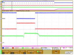
Figure 9-6. Driver PWM operation with feedback
