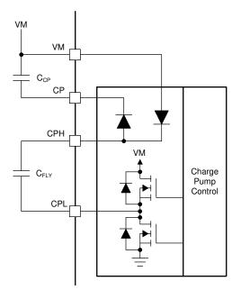
Figure 8-14. DRV8316-Q1 Charge Pump
