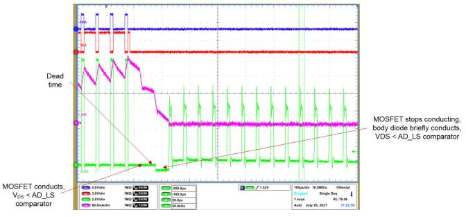
Figure 9-3. Active demagnetization enabled in DRV8316-Q1
