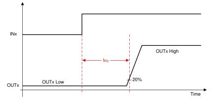
Figure 8-19. Propagation Delay Timing
