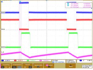
Figure 9-9. Driver delay compensation (1.8 µs)
