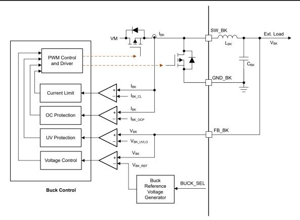
Figure 8-12. Buck Operation and Control Loops
