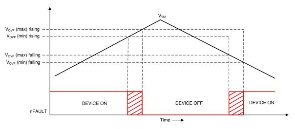
Figure 8-41. Over Voltage Protection
