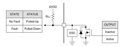
Figure 8-24. Open Drain
