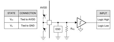
Figure 8-22. Logic-Level Input Pin Structure
