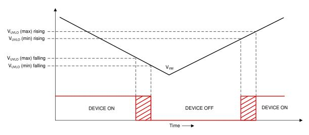
Figure 8-40. VM Supply Undervoltage Lockout
