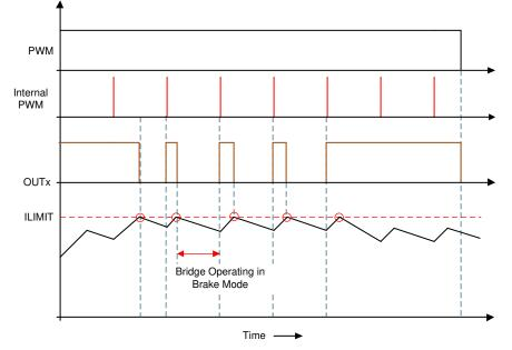
Figure 8-39. Cycle-by-Cycle Current-Limit Operation with 100% PWM Duty Cycle
