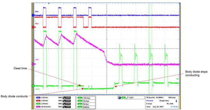
Figure 9-2. Active demagnetization disabled in DRV8316-Q1
