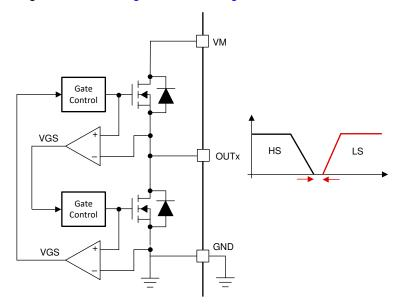
Figure 8-17. Cross Conduction Protection
