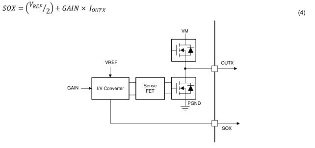
Figure 8-27. Integrated Current Sense Amplifier
