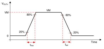
Figure 8-16. Slew Rate Timings
