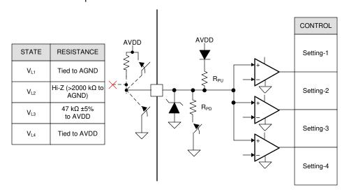
Figure 8-26. Four Level Input Pin Structure
