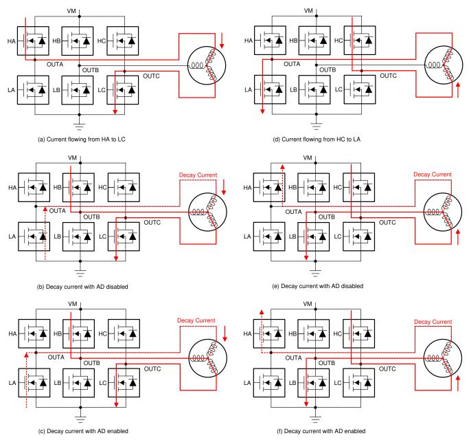
Figure 8-31. ASR in BLDC Motor Commutation
