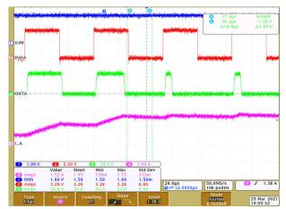
Figure 9-11. Driver PWM with Current Limit
