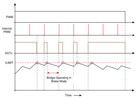
Figure 8-39. Cycle-by-Cycle Current-Limit Operation with 100% PWM Duty Cycle
