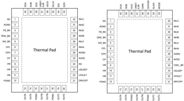
Figure 6-1. DRV8316R 40-Pin VQFN With Exposed Thermal Pad Top View
