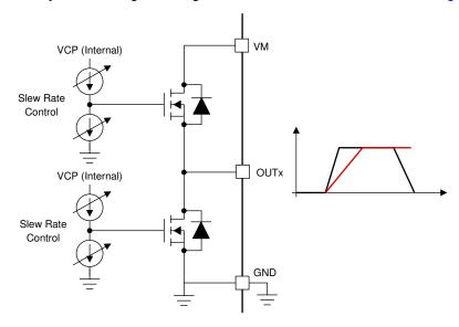
Figure 8-15. Slew Rate Circuit Implementation
