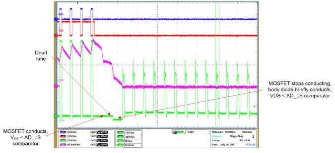
Figure 9-3. Active demagnetization enabled in DRV8316
