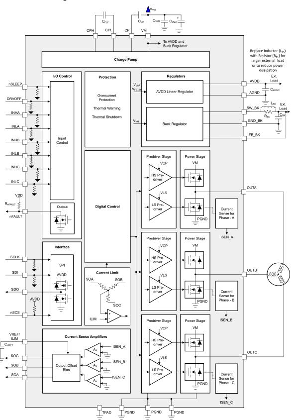
Figure 8-1. DRV8316R Block Diagram
