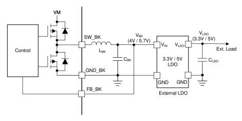
Figure 8-10. Buck Regulator with External LDO
