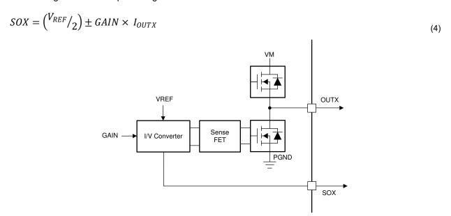
Figure 8-27. Integrated Current Sense Amplifier
