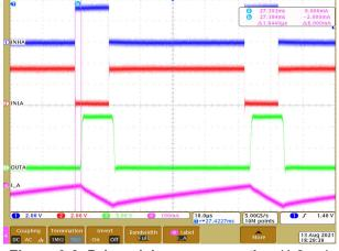
Figure 9-9. Driver delay compensation (1.8 µs)
