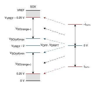
Figure 8-28. Bidirectional Current Sense Output
