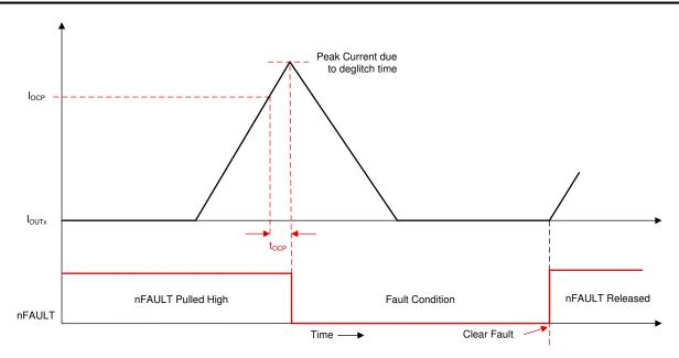
Figure 8-42. Overcurrent Protection - Latched Shutdown Mode
