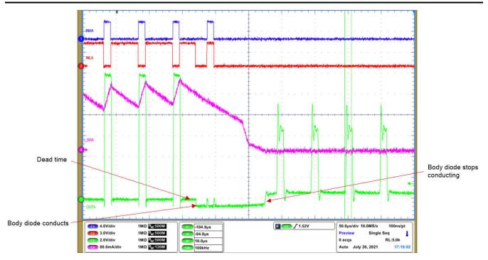
Figure 9-2. Active demagnetization disabled in DRV8316
