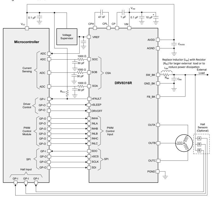
Figure 9-1. Primary Application Schematics
