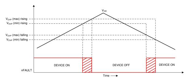
Figure 8-41. Over Voltage Protection
