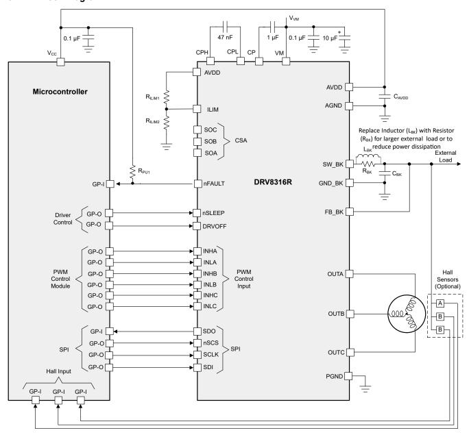
Figure 9-10. Alternate Application - BLDC Motor Control with Current Limit
