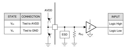
Figure 8-22. Logic-Level Input Pin Structure
