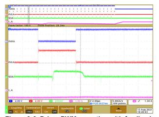
Figure 9-6. Driver PWM operation with feedback
