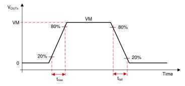
Figure 8-16. Slew Rate Timings
