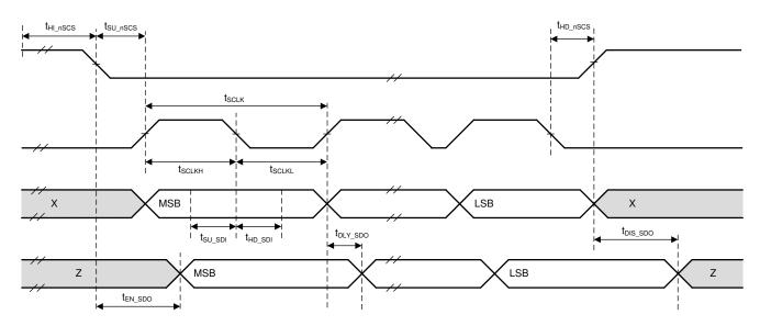
Figure 7-1. SPI Secondary Mode Timings
