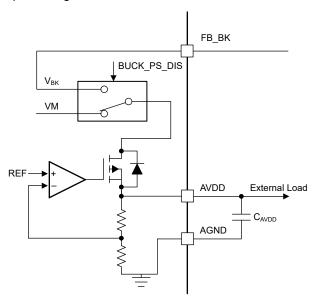
Figure 8-13. AVDD Linear Regulator Block Diagram
