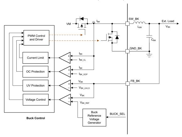
Figure 8-12. Buck Operation and Control Loops
