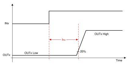
Figure 8-19. Propagation Delay Timing
