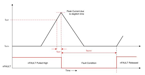
Figure 8-43. Overcurrent Protection - Automatic Retry Mode
