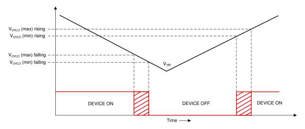
Figure 8-40. VM Supply Undervoltage Lockout
