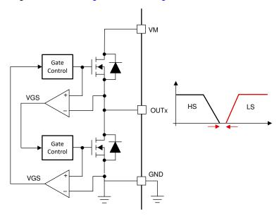
Figure 8-17. Cross Conduction Protection
