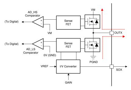
Figure 8-30. Active Demagnetization Operation
