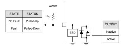
Figure 8-24. Open Drain
