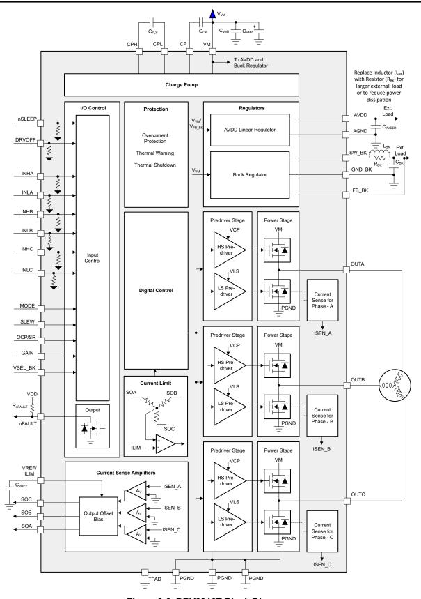
Figure 8-2. DRV8316T Block Diagram
