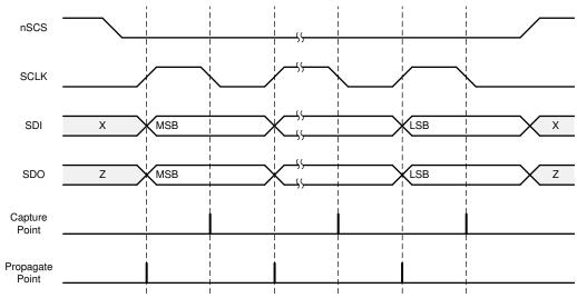
Figure 8-46. SPI Secondary Timing Diagram
