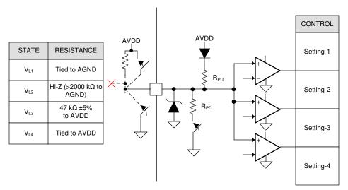
Figure 8-27. Four Level Input Pin Structure
