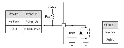
Figure 8-25. Open Drain
