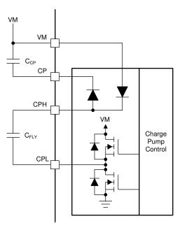
Figure 8-15. DRV8316C-Q1 Charge Pump
