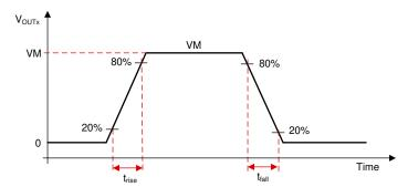
Figure 8-17. Slew Rate Timings
