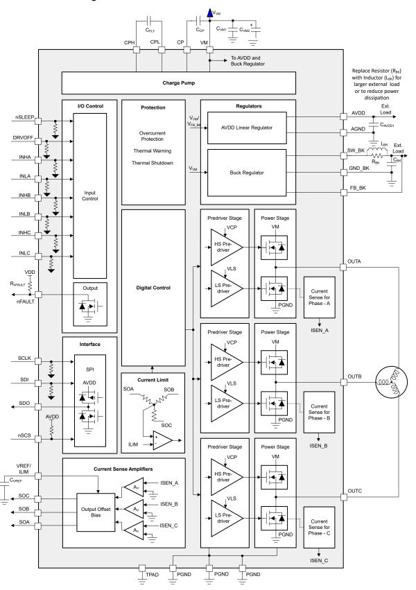
Figure 8-1. DRV8316CR-Q1 Block Diagram
