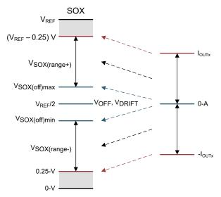
Figure 8-29. Bi-directional Current Sense Linear Region
