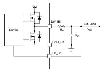
Figure 8-10. Buck (Resistor Mode)
