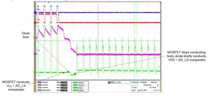
Figure 9-3. Active demagnetization enabled in DRV8316C-Q1
