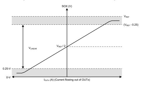
Figure 8-30. IOUTx to CSA Transfer Function
