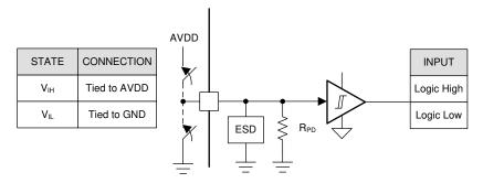
Figure 8-23. Logic-Level Input Pin Structure
