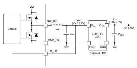
Figure 8-11. Buck Regulator with External LDO
