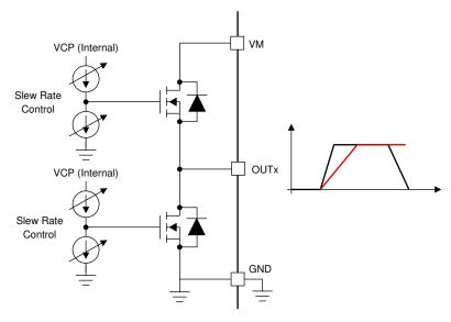
Figure 8-16. Slew Rate Circuit Implementation
