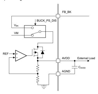
Figure 8-14. AVDD Linear Regulator Block Diagram
