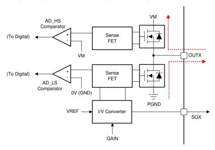
Figure 8-31. Active Demagnetization Operation
