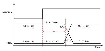
Figure 8-20. Propagation Delay
