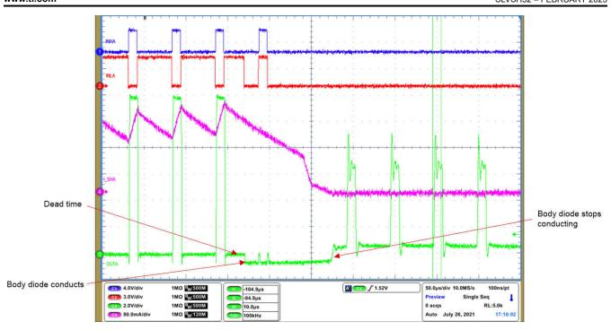
Figure 9-2. Active demagnetization disabled in DRV8316C-Q1
