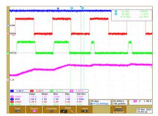
Figure 9-11. Driver PWM with Current Limit
