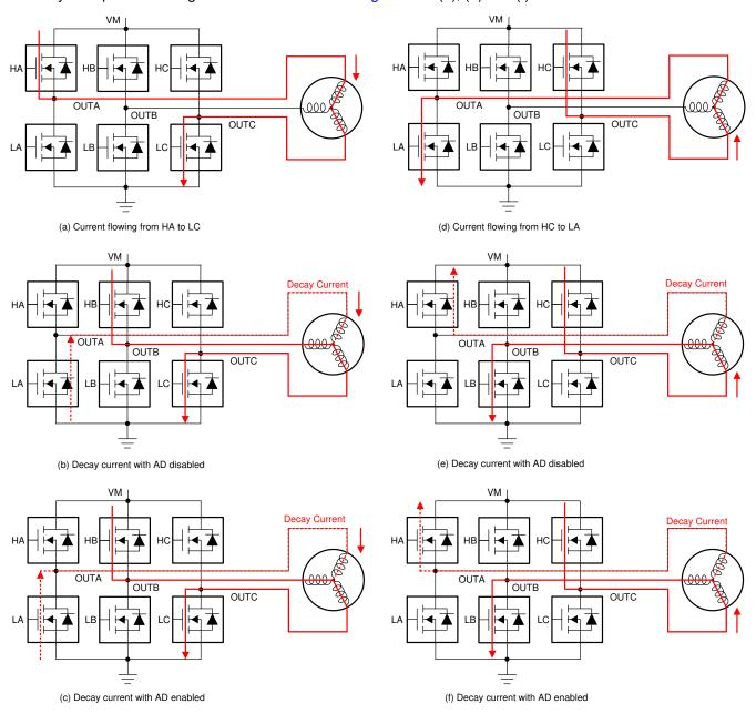
Figure 8-32. ASR in BLDC Motor Commutation
