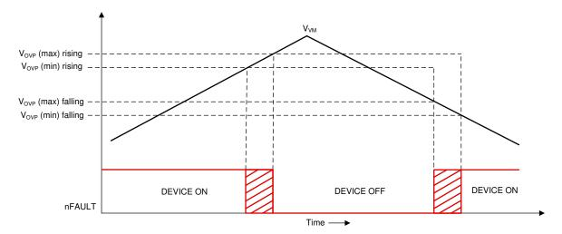
Figure 8-42. Over Voltage Protection
