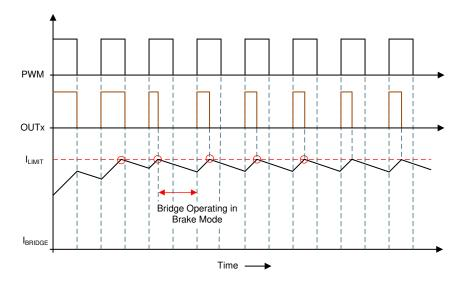
Figure 8-37. Cycle-by-Cycle Current-Limit Operation
