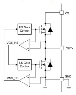
Figure 8-18. Cross Conduction Protection
