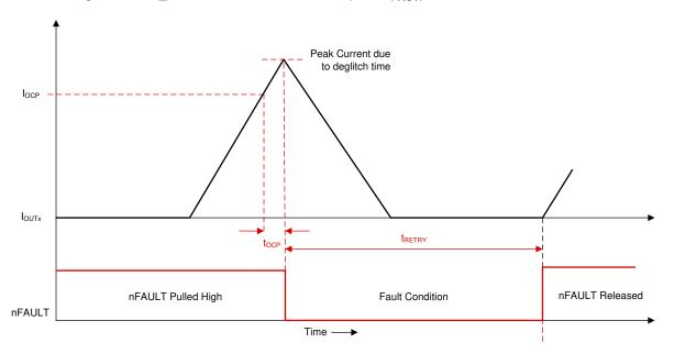
Figure 8-44. Overcurrent Protection - Automatic Retry Mode
