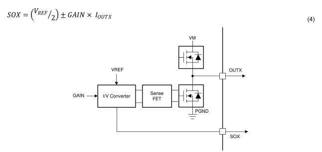
Figure 8-28. Integrated Current Sense Amplifier
