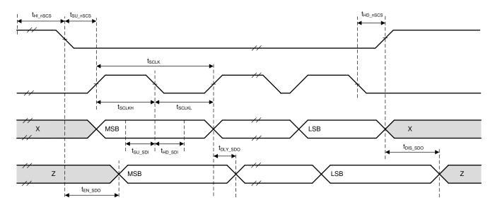
Figure 7-1. SPI Secondary Mode Timings
