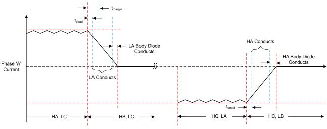
Figure 8-33. Current Waveforms for ASR in BLDC Motor Commutation
