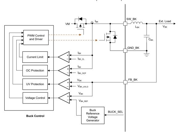
Figure 8-13. Buck Operation and Control Loops
