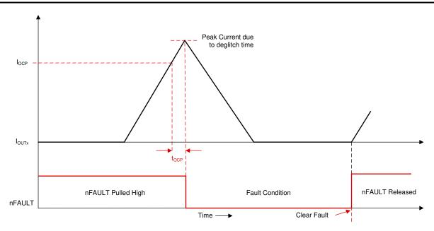
Figure 8-43. Overcurrent Protection - Latched Shutdown Mode
