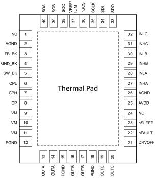
Figure 6-1. DRV8316CR-Q1 40-Pin VQFN With Exposed Thermal Pad Top View
