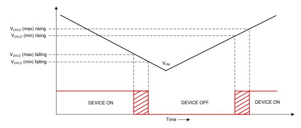
Figure 8-41. VM Supply Undervoltage Lockout
