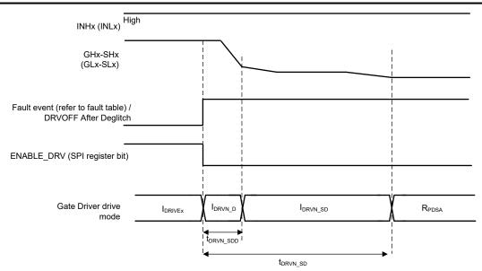
Figure 7-15. Gate Drive Shutdown Sequence
