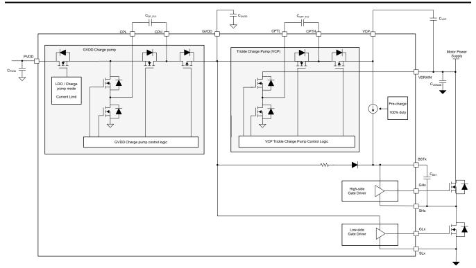
Figure 7-4. DRV8334 Gate Driver Power Supply Architecture
