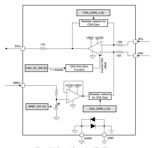
Figure 7-9. Current-Sense Amplifier Diagram
