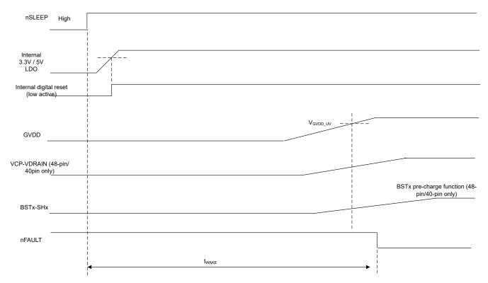
Figure 7-16. Device Power Up Sequence and  $t_{\text{WAKE}}$
