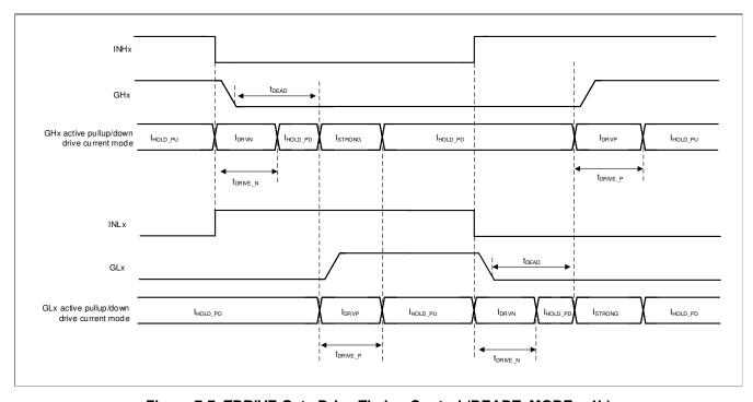
Figure 7-7. TDRIVE Gate Drive Timing Control (DEADT\_MODE = 1b)
