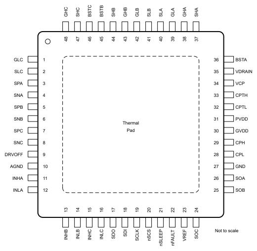
Figure 5-1. DRV8334 Package 48-Pin HTQFP With Exposed Thermal Pad Top View
