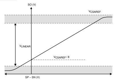
Figure 7-10. Unidirectional Current-Sense Output
