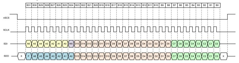
Figure 7-17. SPI Format - 32-bit frame (SPI\_CRC\_EN = 1b)
