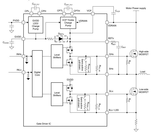
Figure 7-5. Gate Driver Architecture
