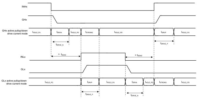
Figure 7-6. TDRIVE Gate Drive Timing Control (DEADT\_MODE = 0b)
