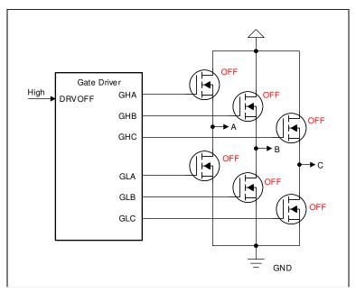
Figure 7-14. DRVOFF Gate Driver Output State
