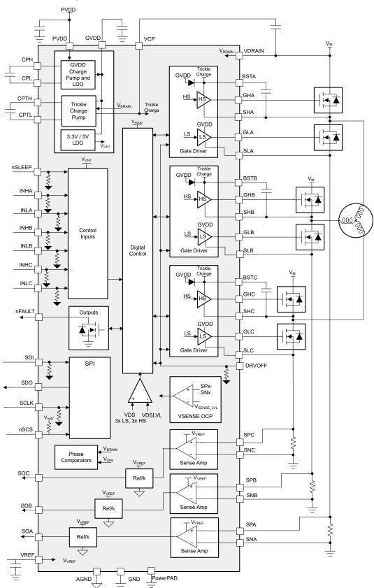
Figure 7-1. Block Diagram of DRV8334
