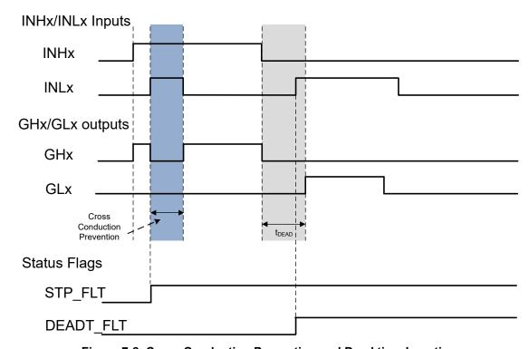
Figure 7-8. Cross Conduction Prevention and Dead time Insertion
