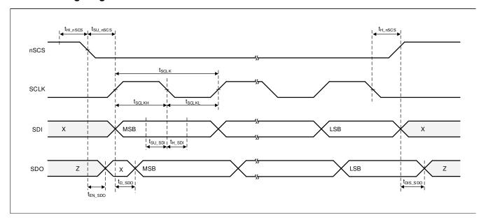
Figure 6-1. SPI Slave Mode Timing Diagram
