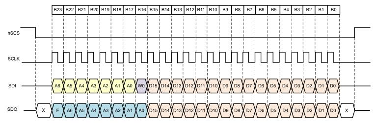
Figure 7-18. SPI Format - 24-bit frame (SPI\_CRC\_EN = 0b)
