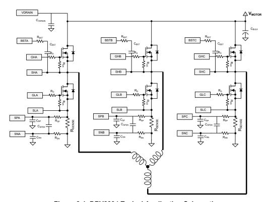
Figure 8-1. DRV8334 Typical Application Schematic
