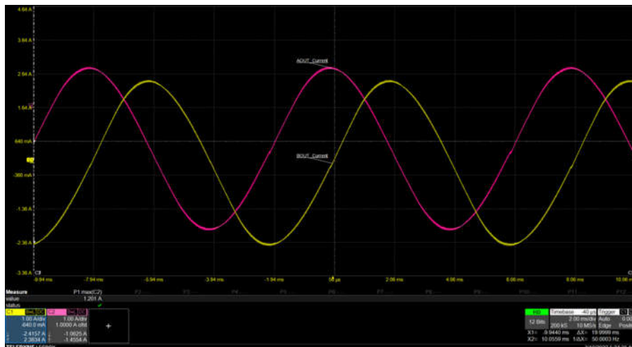
Figure 7-20. Coil Current Waveform with Silent Step Decay
