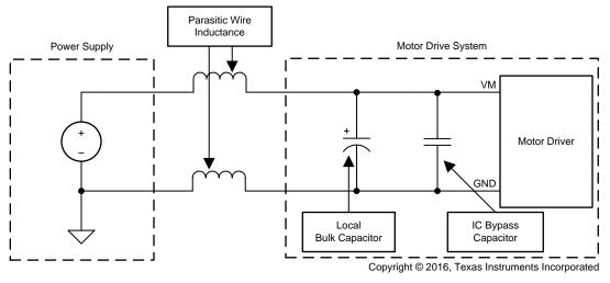
Figure 7. Bulk Capacitor
