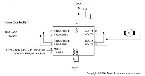
Figure 5. Parallel Mode Connections
