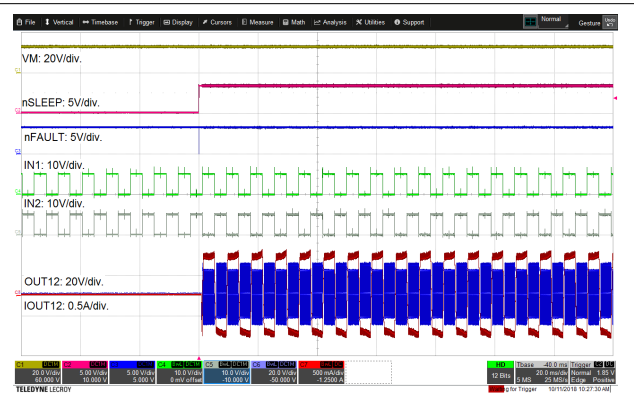
Figure 8-6. Device Power-up with nSLEEP
