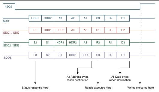
Figure 7-18. SPI Frame With Three DRV8873S-Q1 Devices
