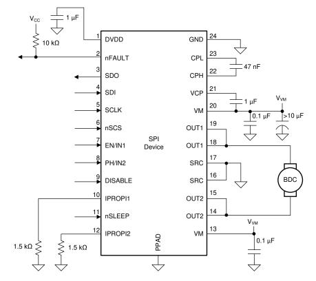
Figure 8-1. Typical Application Schematic
