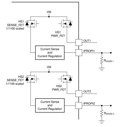
Figure 7-5. Current-Sense Block Diagram
