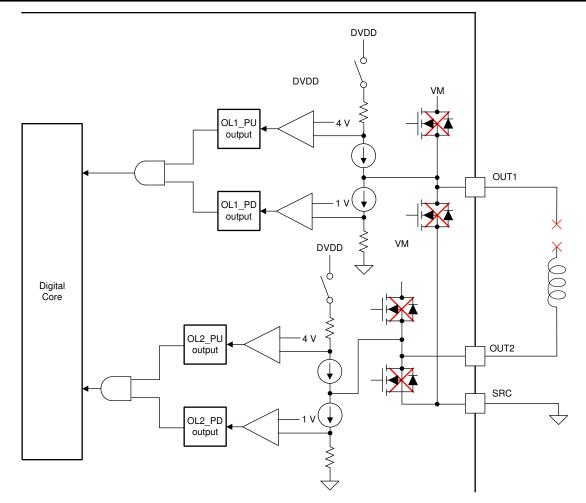
Figure 7-12. Open-Load Detection Circuit
