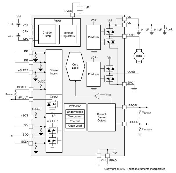
Figure 7-2. SPI Device Block Diagram
