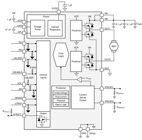
Figure 7-1. Hardware Device Block Diagram
