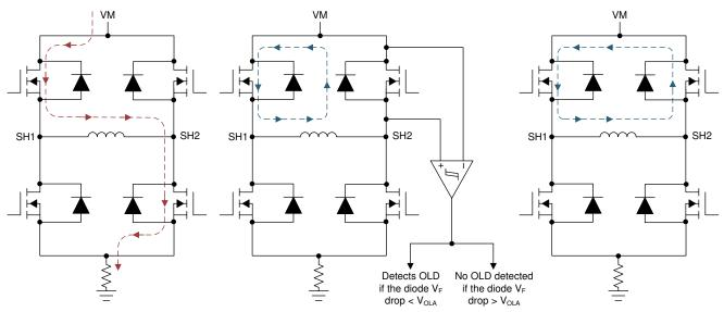
Figure 7-13. Open-Load Active Mode Circuit
