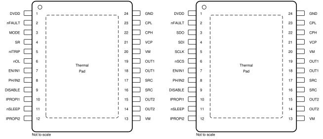
Figure 5-1. DRV8873H-Q1 PWP PowerPAD Package Figure 5-2. DRV8873S-Q1 PWP PowerPAD Package 24-Pin HTSSOP Top View 24-Pin HTSSOP Top View
