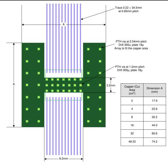
Figure 8-2. PCB Model (4-Layer PCB Shown, 2-Layer PCB Has No Vias)
