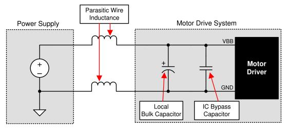
Figure 9-1. System Supply Parasitics Example
