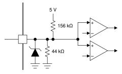
Figure 7-8. PMODE Tri-Level Input
