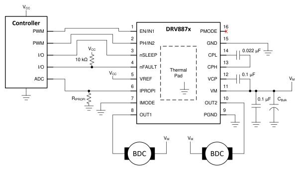
Figure 8-15. Typical Application Schematic
