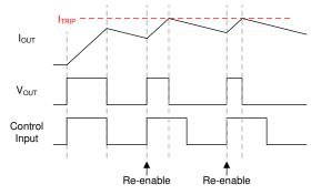
Figure 7-4. Cycle-By-Cycle Current Regulation
