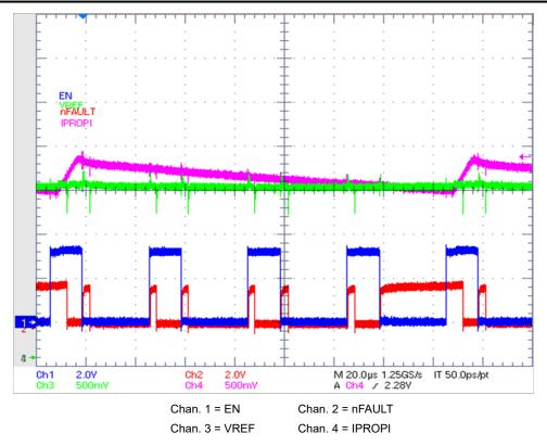
Figure 7-6. nFAULT Pin When  $V_{IPROPI} > V_{VREF}$  with PH/EN Mode and PWM Signal on EN Pin
