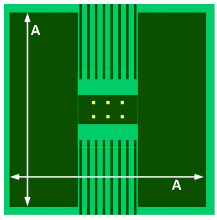
Figure 8-2. HTSSOP PCB model top layer
