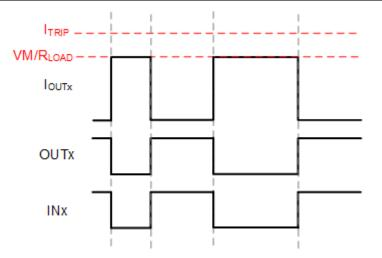
Figure 7-3. Resistive Load Connected to VM, Cycle-by-cycle control, I<sub>TRIP</sub> is higher than VM/R<sub>LOAD</sub>.
