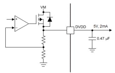
Figure 7-10. Linear Voltage Regulator Block Diagram
