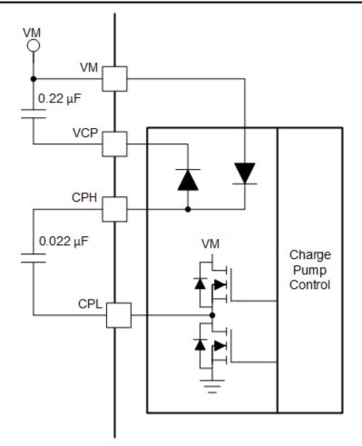
Figure 7-9. Charge Pump Block Diagram
