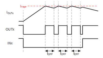
Figure 7-4. Inductive Load Connected to VM, fixed off-time current chopping
