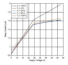
Figure 6-1. Sleep Current over Supply Voltage
