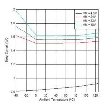
Figure 6-2. Sleep Current over Temperature
