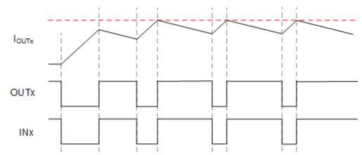
Figure 7-5. Inductive Load Connected to VM, Cycle-by-cycle control
