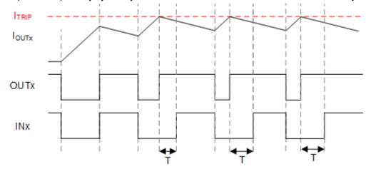
Figure 7-6. Inductive Load Connected to VM, Cycle-by-cycle control, T has to be less than T<sub>OFF</sub> of the DRV8955.
