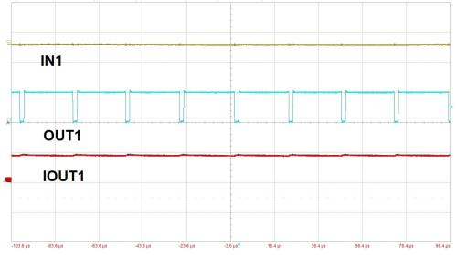
Figure 8-2. Current Regulation with VM-connected Load
