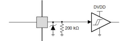
Figure 7-11. Logic-level Input Pin Diagram
