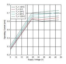
Figure 6-3. Operating Current over Supply Voltage
