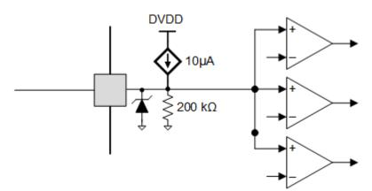
Figure 7-12. Quad-Level Input Pin Diagram
