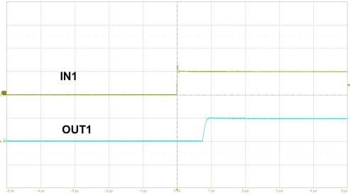
Figure 8-3. Input-to-Output Propagation Delay
