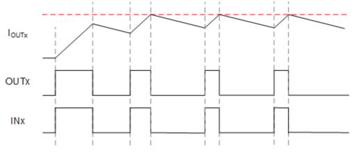
Figure 7-7. Inductive Load Connected to ground, Cycle-by-cycle control
