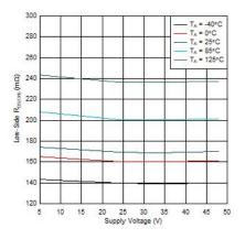
Figure 6-5. Low-Side  $R_{\text{DS(ON)}}$  over Supply Voltage (MODE = 0 or 330k to GND)
