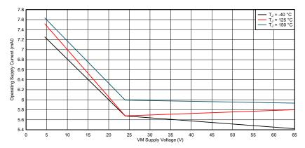
Figure 6-4. Operating supply current, VCC = DVDD
