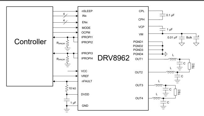
Figure 8-8. Driving two TECs
