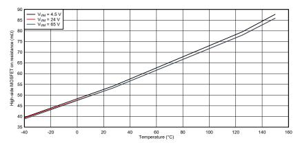
Figure 6-5. High-side FET on resistance
