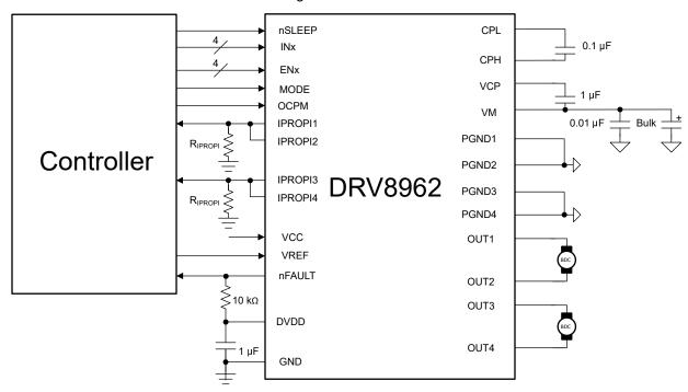
Figure 8-6. Driving two Brushed-DC Motors with DRV8962
