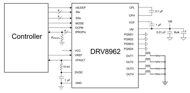
Figure 8-1. Driving Solenoids with DRV8962
