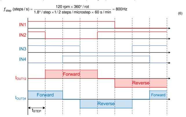
Figure 8-5. Example 1/2 Stepping Operation
