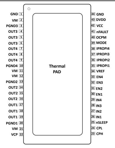
Figure 5-2. DDV Package, Top View
