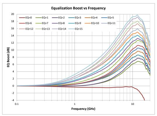
Figure 6-1. Typical EQ Boost vs Frequency
