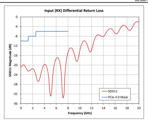
Figure 6-3. Typical RX Differential Return Loss
