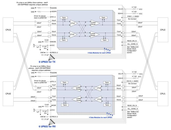
Figure 8-2. Simplified Schematic for UPI 2x2 cross-point mux for x24Lane Configuration in SMBus/I<sup>2</sup>C Master Mode
