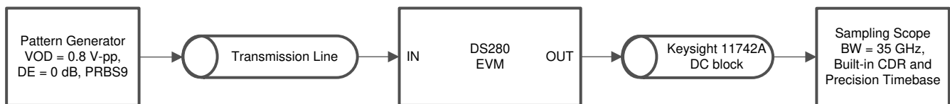
Figure 9-16. 10 in input channel and minimal output channel test setup
