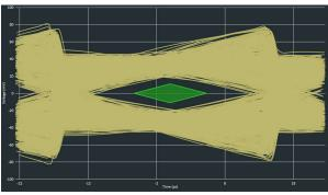
Figure 8-4. PCle 5.0 link Baseline Setup Without Redriver Eye Diagram Using SigTest
