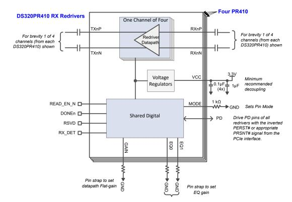
Figure 8-2. Simplified Schematic for PCle x16 Lane Configuration in Pin mode
