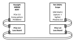
Figure 8-3. PCIe 5.0 Link Baseline Setup Without Redriver the Link Elements
