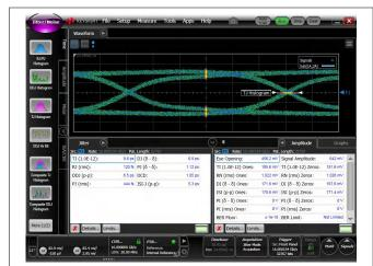
Figure 6-3. Through Baseline Calibration Trace (no redriver)
