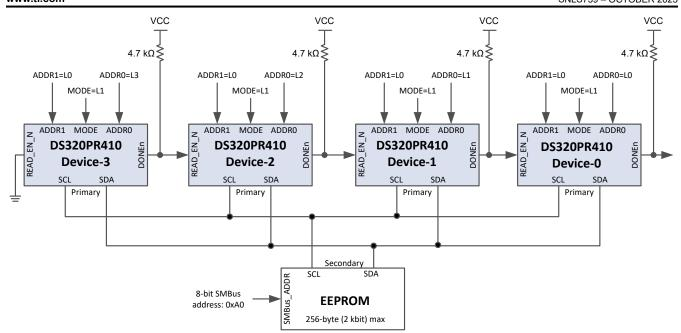
Figure 7-1. Daisy Chain Four DS320PR410 Devices to Read from Single EEPROM
