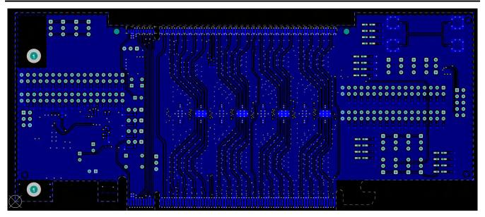
Figure 8-8. Layout Example: TI PCle 5.0 Riser Card Using DS320PR410 With CEM Connectors - Bottom Layer
