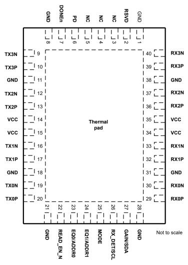
Figure 5-1. RNQ Package, 40-Pin WQFN (Top View)
