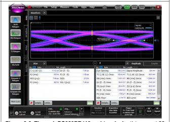
Figure 6-6. Through DS320PR410 and (equivalent) traces at 32 Gbps with EQ = 0 (4 dB)
