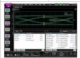
Figure 6-5. Through Baseline Calibration Trace (no redriver)
