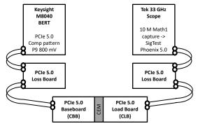
Figure 8-5. PCle 5.0 Link Baseline Setup Without Redriver the Link Elements
