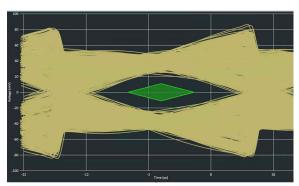
Figure 8-6. PCle 5.0 link Baseline Setup Without Redriver Eye Diagram Using SigTest
