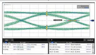
Figure 6-6. Through DS320PR810 (7 dB Loss and DUT EQ = 0)
