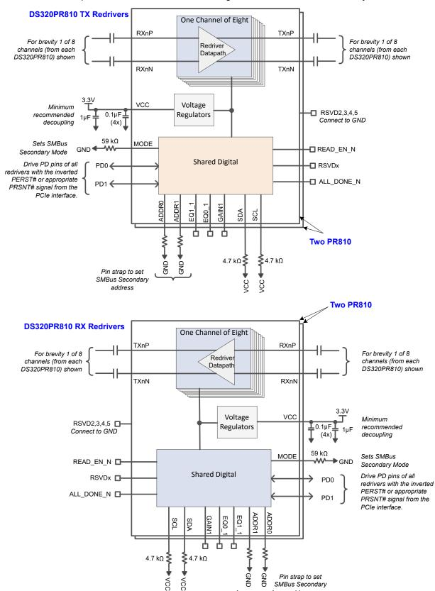
Figure 8-4. Simplified Schematic for PCle x16 Lane Configuration in SMBus/I<sup>2</sup>C Secondary mode
