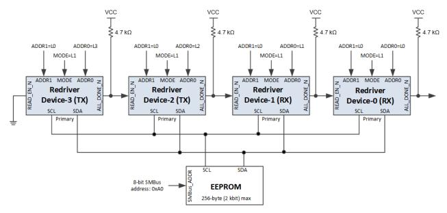
Figure 7-1. Daisy Chain Four DS320PR810 Devices to Read from Single EEPROM in x16 Configuration
