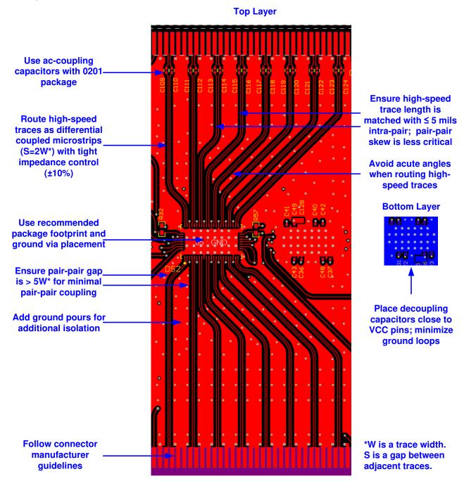
Figure 10-1. DS320PR810 Layout Example - Sub-Section of a PCle Riser Card With CEM Connectors
