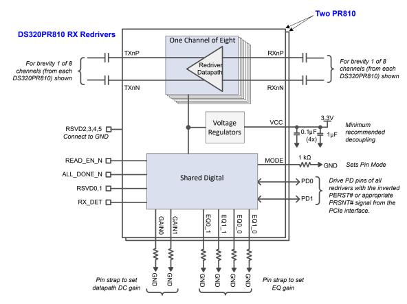
Figure 8-2. Simplified Schematic for PCle x16 Lane Configuration in Pin mode
