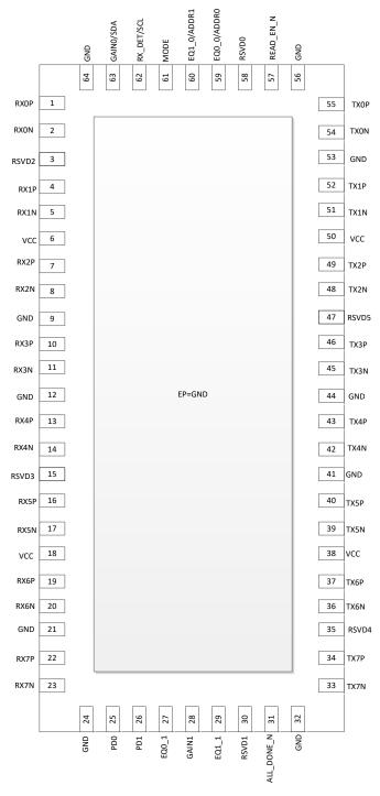
Figure 5-1. NJX Package, 64-Pin WQFN (Top View)
