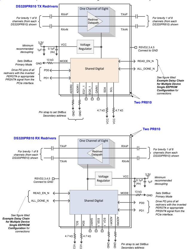
Figure 8-3. Simplified Schematic for PCle x16 Lane Configuration in SMBus/I<sup>2</sup>C Primary mode
