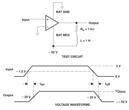
Figure 2. Test Circuit and Voltage Waveforms, Each Driver
