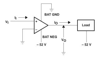
Figure 1. Generalized Test Circuit, Each Driver
