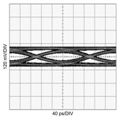
Figure 37. Equalized Signal (10m 24AWG PCle Cable, 5Gbps, PRBS7)
