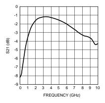
Figure 3. Typical Equalizer Transfer Function
