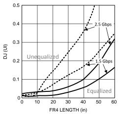
Figure 6. Residual Deterministic Jitter vs. FR4 Length
