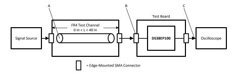
Figure 1. Transient Test Setup Diagram
