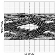
Figure 33. Unequalized Signal (10m 24AWG PCle Cable, 2.5Gbps, PRBS7)
