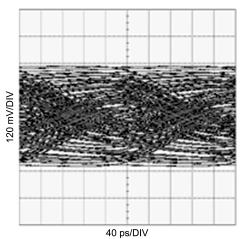
Figure 36. Unequalized Signal (10m 24AWG PCle Cable, 5Gbps, PRBS7)
