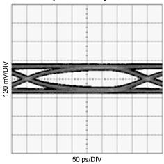
Figure 34. Equalized Signal (10m 24AWG PCle Cable, 2.5Gbps, PRBS7)
