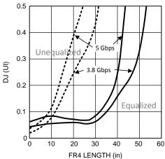
Figure 5. Residual Deterministic Jitter vs. FR4 Length
