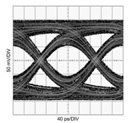
Figure 38. Equalized Signal (Zoom) (10m 24AWG PCle Cable, 5Gbps, PRBS7)
