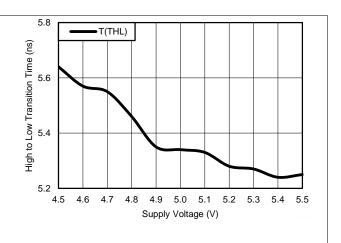
ow to High Transition Time Figure 2. Typical Driver Output High to Low Transition Time vs Supply Voltage
