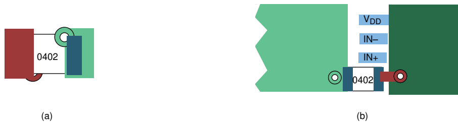
Figure 11-7. Typical Decoupling Capacitor Layouts
