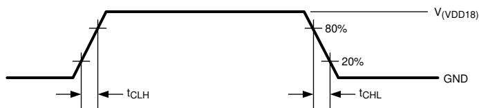
Figure 5-1. LVC MOS Transition Times
