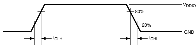
Figure 6-1. LVCMOS Transition Times
