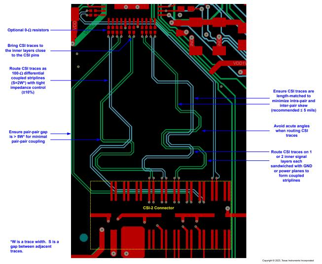
Figure 8-19. Example Routing of CSI-2 Traces
