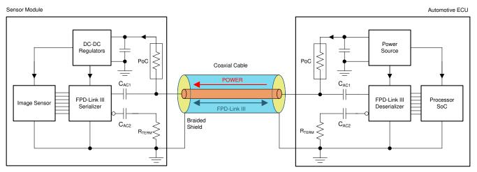
Figure 8-1. Power-over-Coax (PoC) System Diagram
