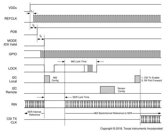
Figure 8-15. Power-Up Sequencing With Synchronous Clocking Mode
