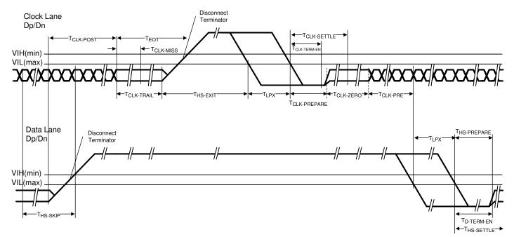
Figure 6-6. Switching the Clock Lane between Clock Transmission and Low-Power Mode
