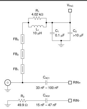
Figure 8-2. Example Recommended PoC Network for a "4G" FPD-Link III
