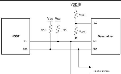
Figure 7-18. Serial Control Bus Connection
