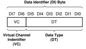
Figure 7-10. CSI-2 Data Identifier Structure
