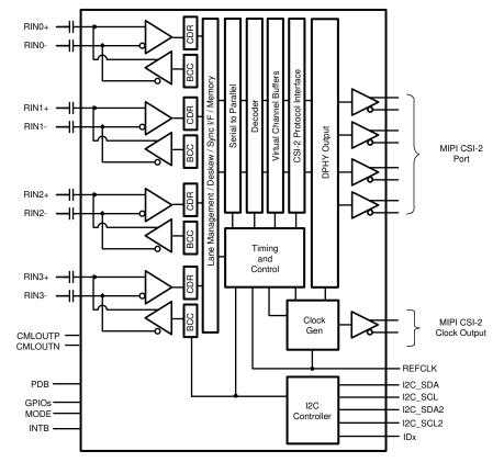
Figure 7-1. Functional Block Diagram
