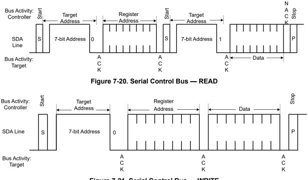
Figure 7-21. Serial Control Bus — WRITE
