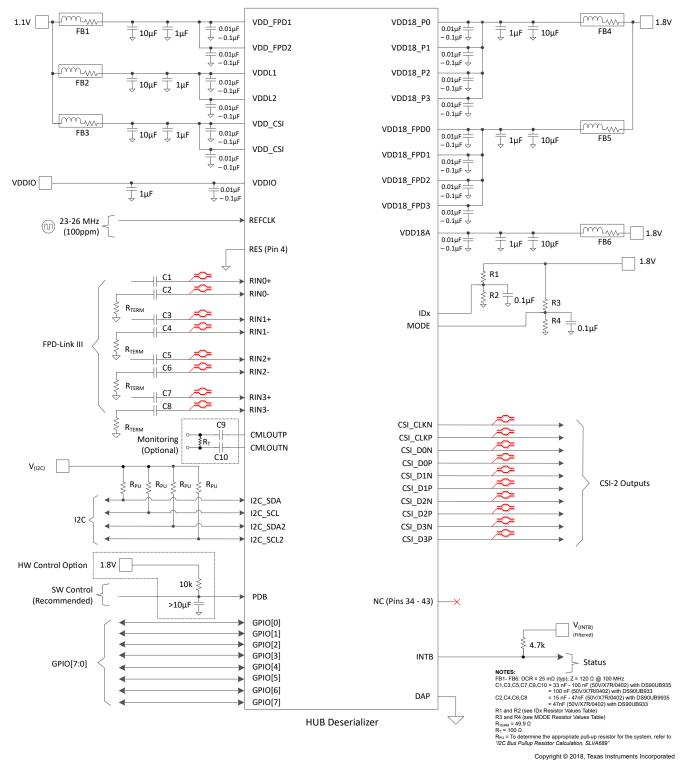
Figure 8-4. Typical Connection Diagram (Coaxial)
