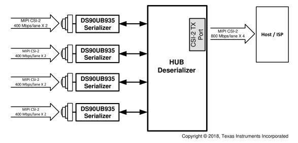
Figure 8-12. Four DS90UB935-Q1 Sensor Data Onto CSI-2
