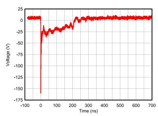
Figure 8-2. +8-kV Clamped IEC Waveform
